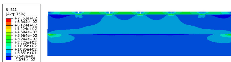
Figure 5.14: Exemple of the periodic model of \rho_p = 0.2 and \rho_c = 0.3
