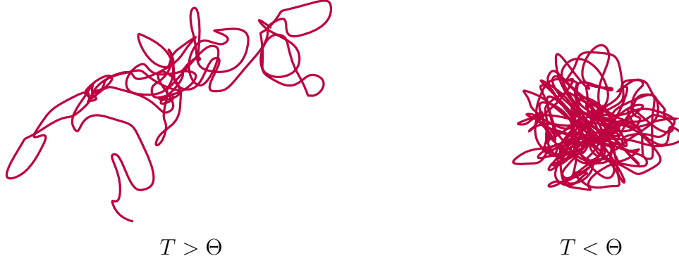
Figure 1.6: Coil (left) and globule (right) configurations of a polymer chain, obtained by varying the solvent temperature across the so-called theta temperature \Theta .
