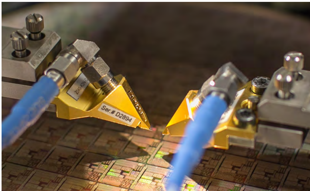
Figure F.3: GSG probes on B5T HBT multi-project wafer for pulsed RF measurement on PA200 prober, IMS Bordeaux
