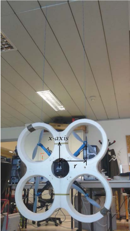
(a) Supporting wires position for x and y axis
