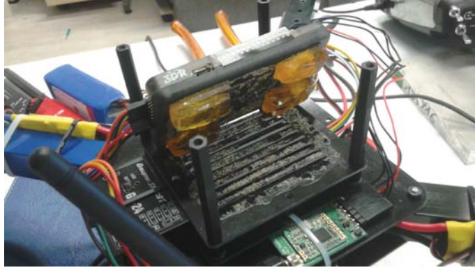
Figure 5.3.1: Used vibration dampening gel
