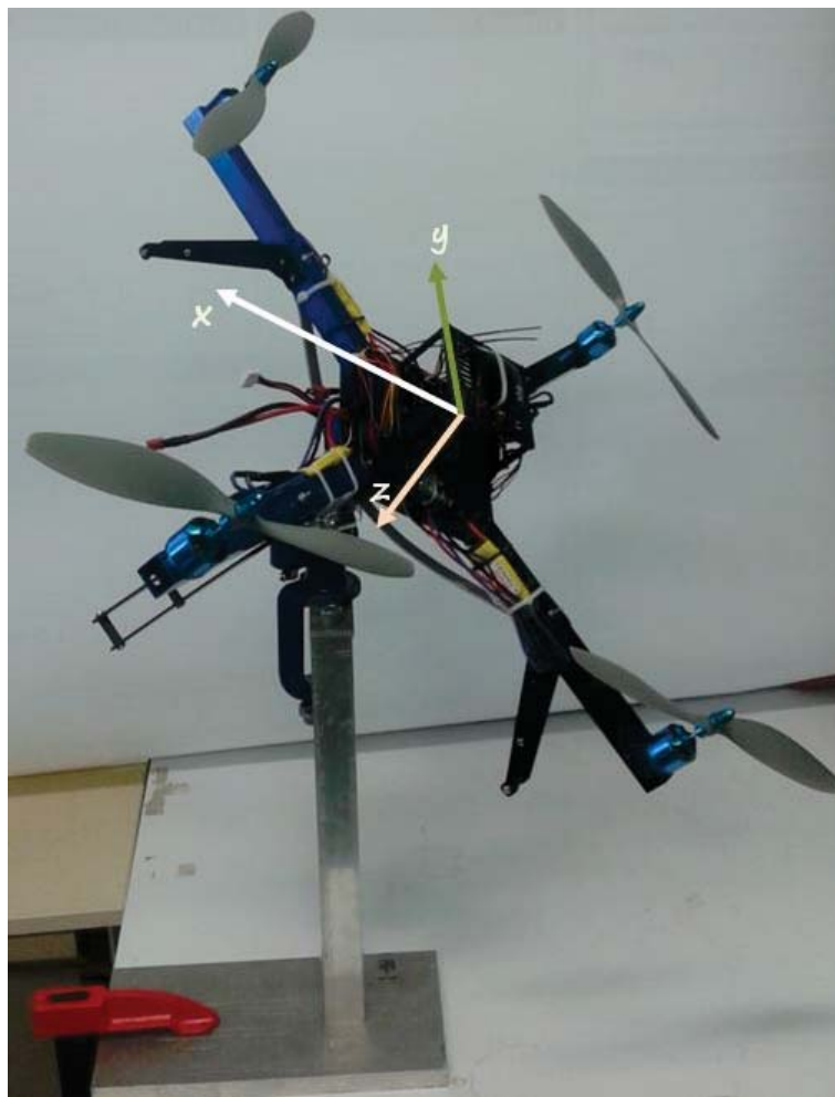
Figure 5.2.1: Test-bench DIY Quad equipped with the APM2.6 autopilot
