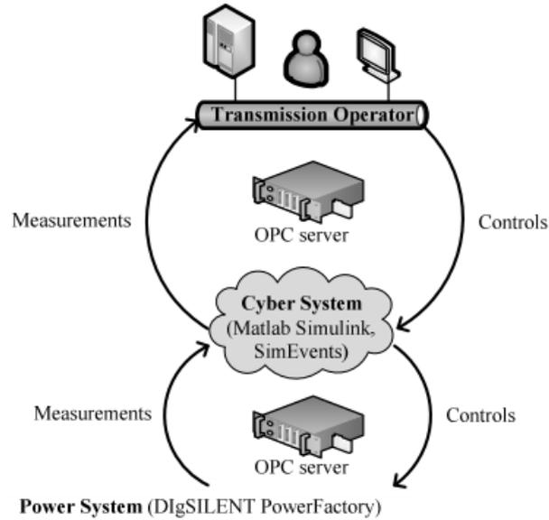
Figure II:10 Cyber-physical power system architecture (Stefanov and Liu 2012)
