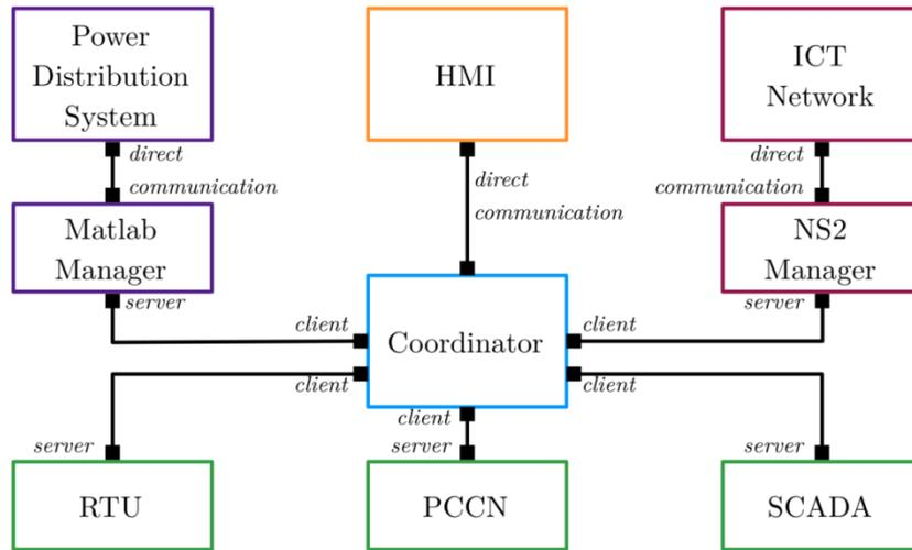
Figure II:9 Cosimulator Architecture
