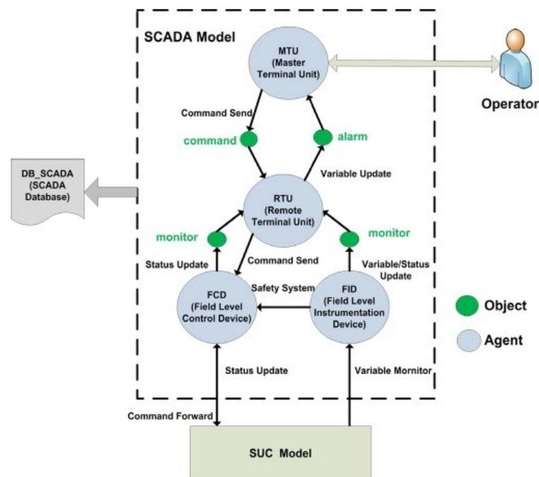
Figure II:5 Overall SCADA model (Nan, Eusgeld and Kröger 2013)
