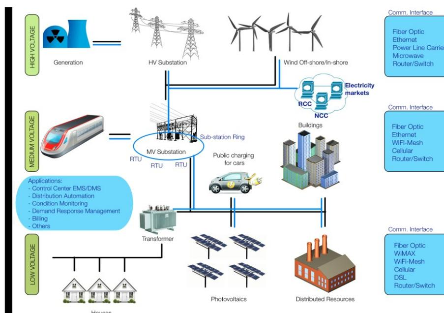
Figure I:6 Electric power system and Control Network
