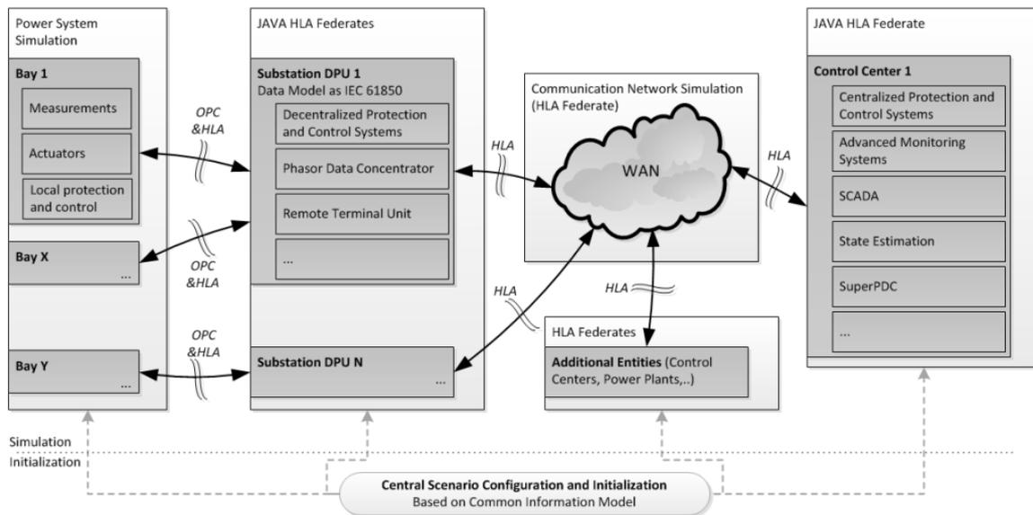
Figure II:11 Hybrid simulator components (Müller, et al. 2012)
