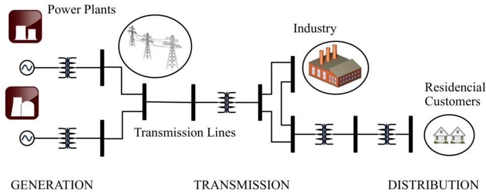
Figure I:3 Typical structure of Electric Power Systems
