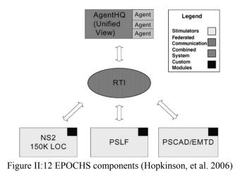
to help components interaction. An RTI is used to control the simulation synchronization and the routing of communication between EPOCHS components.
