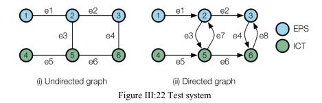
The graphs presented in Figure III:22 will be used to exemplify the elaboration of the adjacency matrices.
