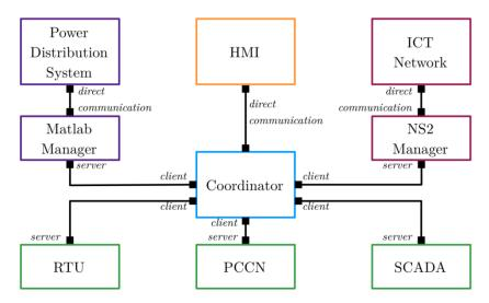
Figure II:9 Cosimulator Architecture
