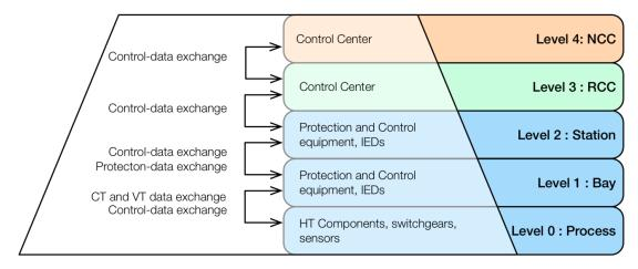
Figure I:5 Hierarchical conceptual levels of EPS (Tranchita, Hadjsaid, et al. 2010)
