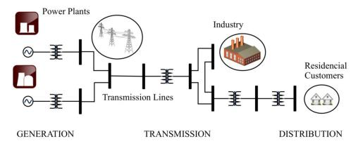
Figure I:3 Typical structure of Electric Power Systems
