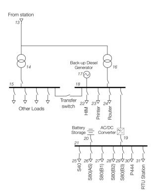
Figure V:5 Auxiliary Control supply system
