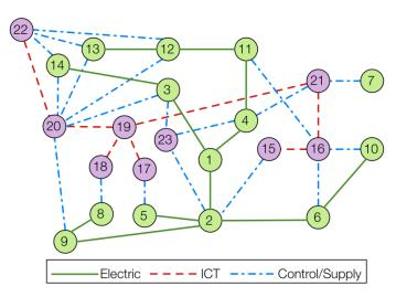
Figure IV:2 Undirected Graph for the 14-bus Test system
