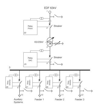
Figure V:3 Substation diagram including Control devices
