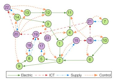
Figure IV:3 Directed Graph for the 14-bus Test system
