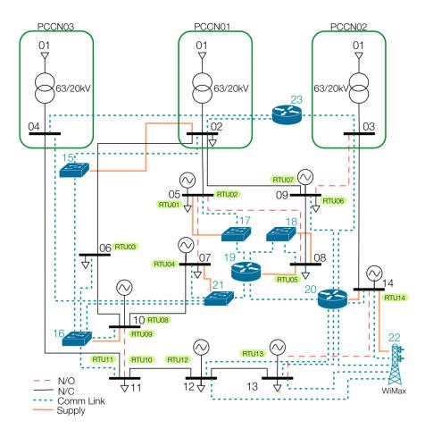
Figure IV:1 Complete 14-Bus Tests System
