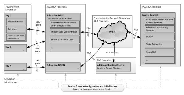
Figure II:11 Hybrid simulator components (Müller, et al. 2012)
