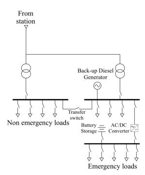
Figure I:8 Auxiliary systems power supply
