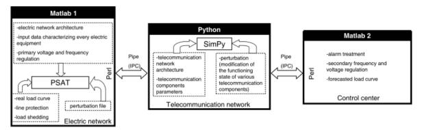
Figure II:8 Combined Simulator (Rozel, et al. 2008)
