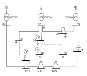
Figure III:10 G2ELAB 14-Bus System
