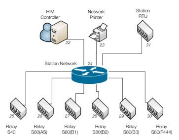
Figure V:4 Substation Communication Network
