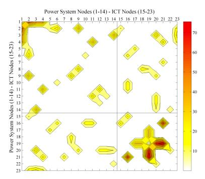
Figure IV:15 Edges Betweenness Centrality - Undirected Graph
