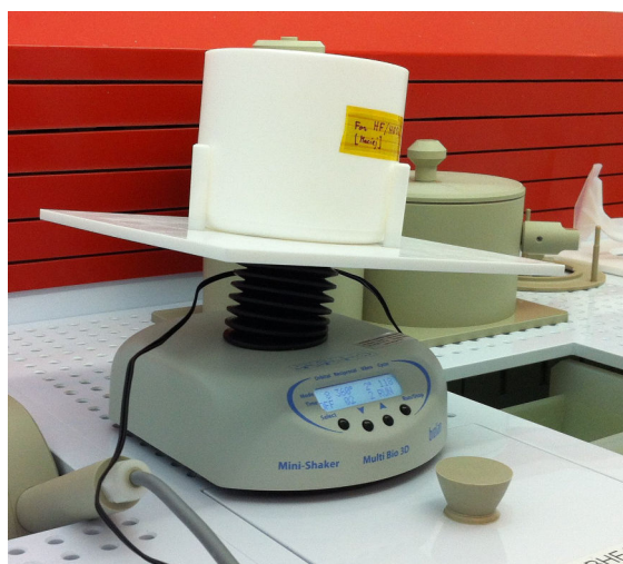
Figure 4.19: Agitation setup for isotropic silicon etching - The Agitator [205] allows quasi-random movement of the etching baker. This is needed to improve aspect ratio of etched structures without introducing asymmetrical effects that can be caused by classical monotonic agitation systems. The agitator from BIOSAN was adapted to the need of etching station by replacing original platform by a PTFE one to provide holder for the etching baker 1 .
