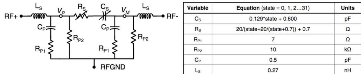
Figure 2.3: Equivalent circuit model schematic of DTC
