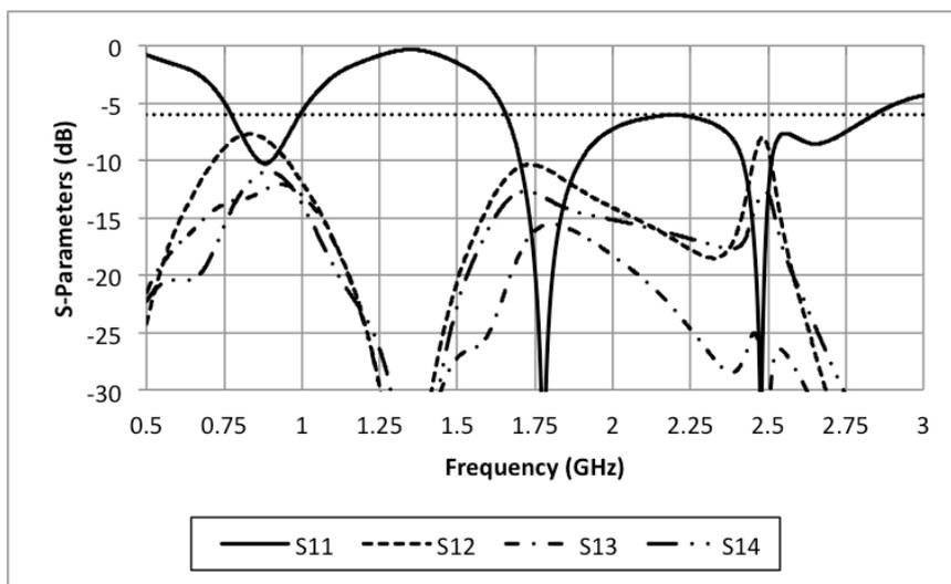
Figure 3.22: Simulated S-parameters of the proposed antenna
