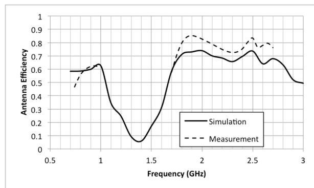
Figure 3.26: Simulated and measured efficiency of the prototype.
