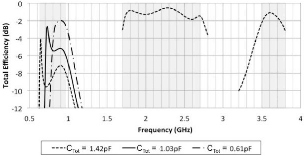
Figure 3.32: Simulated total efficiencies of proposed antenna.
