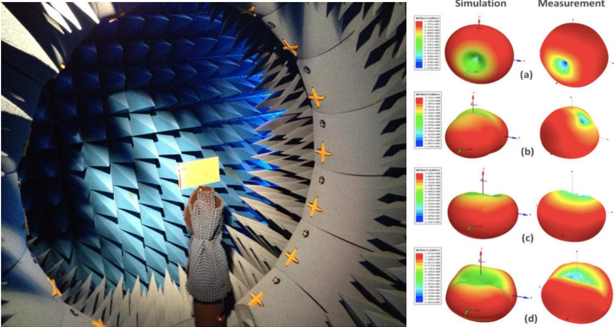
Figure 3.16: Simulated and measured 3D radiation pattern at (a) 700 MHz, (b) 1710 MHz, (c) 2170 MHz, (d) 2700 MHz
