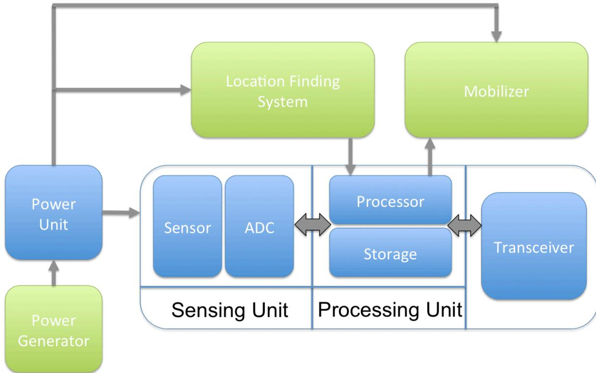
Figure 1.13: Architecture of typical wireless sensor nodes
