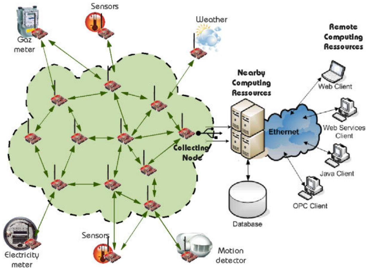
Figure 1.12: Classical structure of wireless sensor networks
