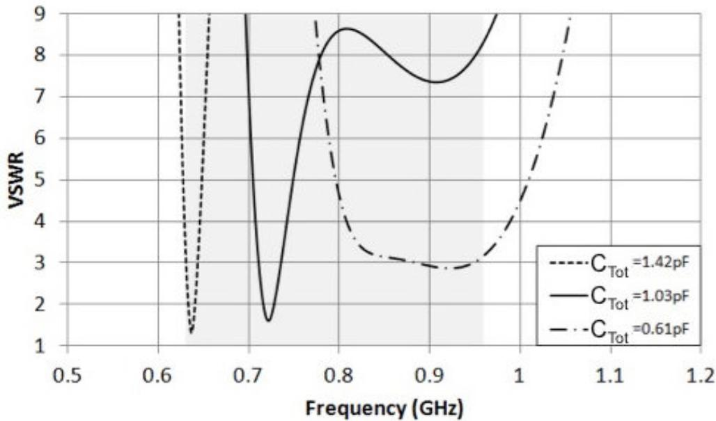
Figure 3.30: Simulated VSWR of proposed antenna at the low frequency bands
