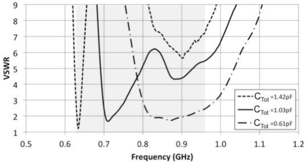
Figure 3.35: Measured antenna VSWR in the low frequency band
