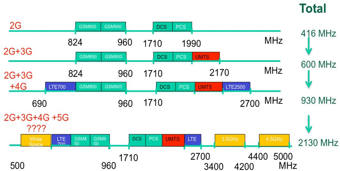
Figure 1.11: Frequency spectrum requirements for future standard antenna
