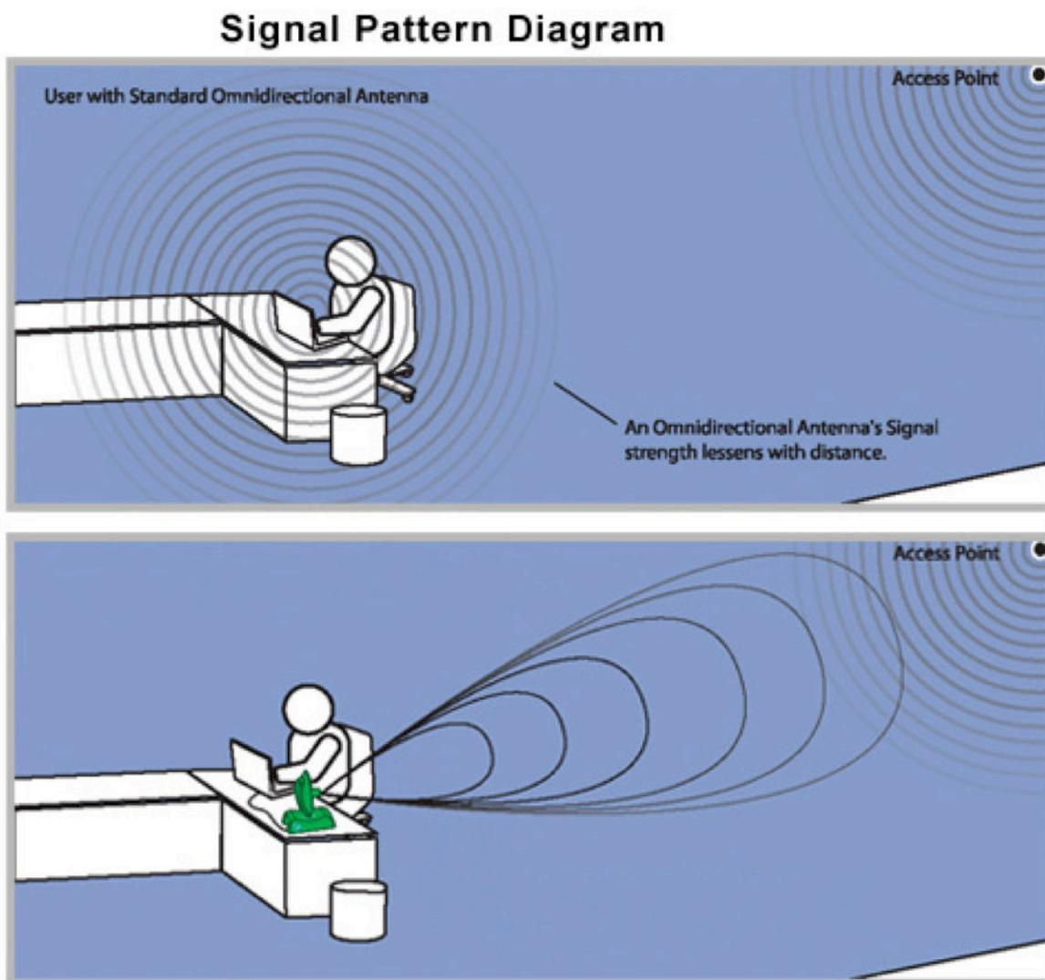
Figure 1.14: Comparison between omnidirectional and directional antennas.
