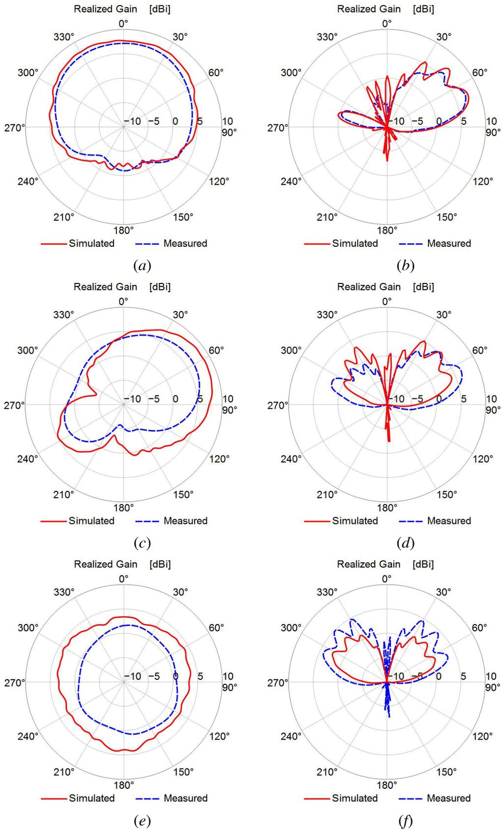
Figure 4.11: Comparison between simulated and measured realized gain pattern of C2C antenna system. (a) Conf.  $C_{11}$  at  $\theta = 68^\circ$ , (b) conf.  $C_{11}$  at  $\varphi = 0^\circ$ , (c) conf.  $C_{21}$  at  $\theta = 68^\circ$ , (d) conf.  $C_{21}$  at  $\varphi = 0^\circ$ , (e) conf.  $C_{31}$  at  $\theta = 68^\circ$ , and (f) conf.  $C_{31}$  at  $\varphi = 0^\circ$ .
