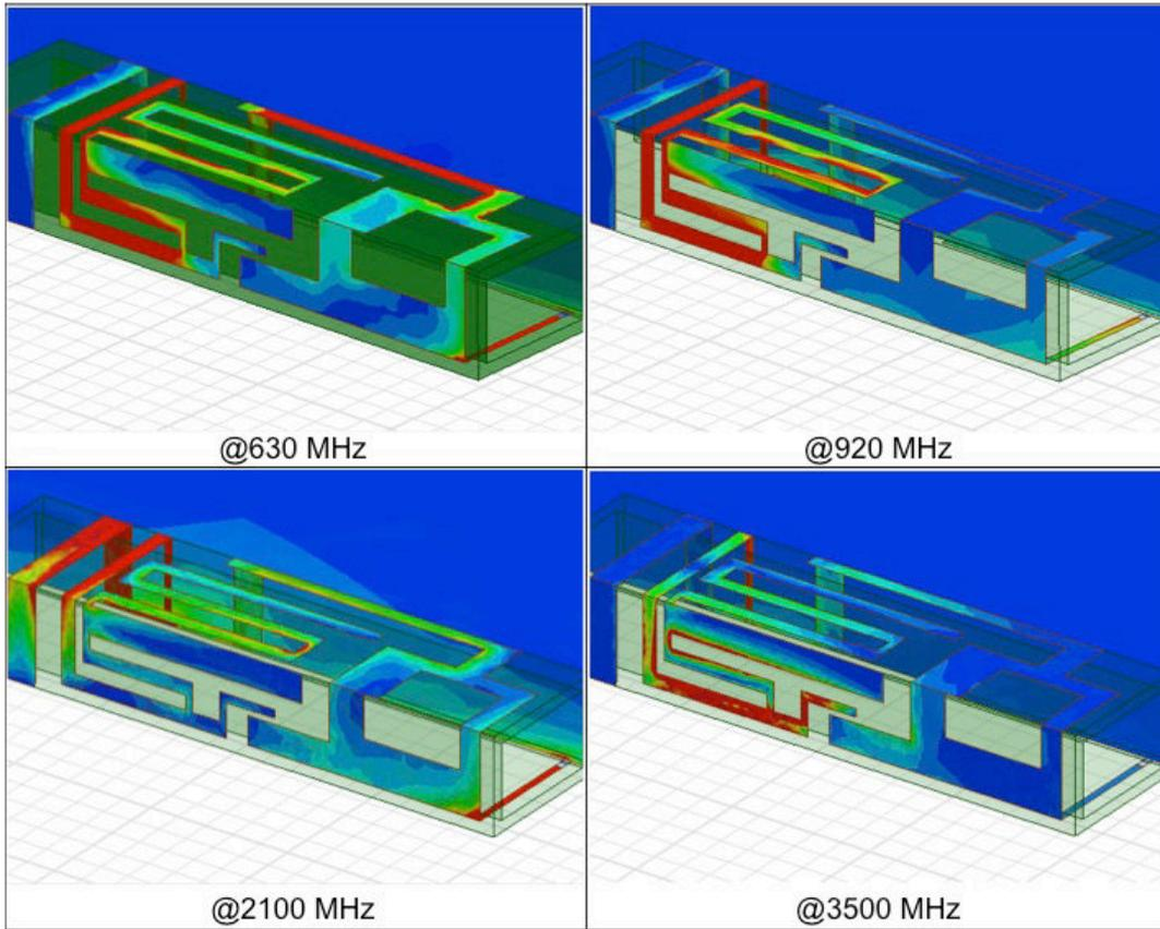
*Figure 3.33: Simulated current distribution at different frequencies.*
