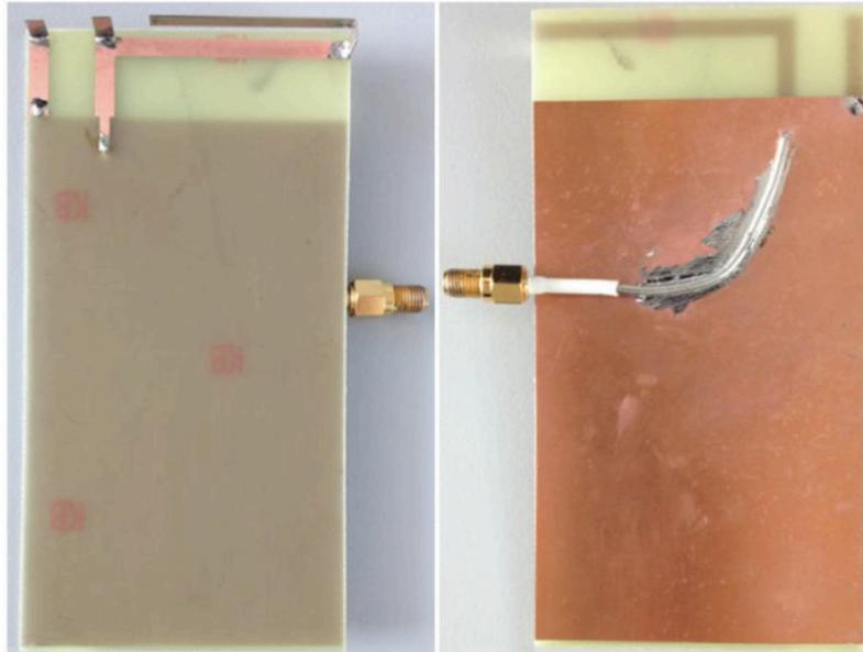
Figure 3.14: The prototype of the proposed antenna on a FR-4 Epoxy.
