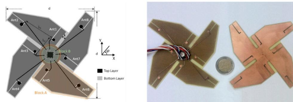
Figure 4.2: Geometry of compact switched-beam steering antenna [2]
