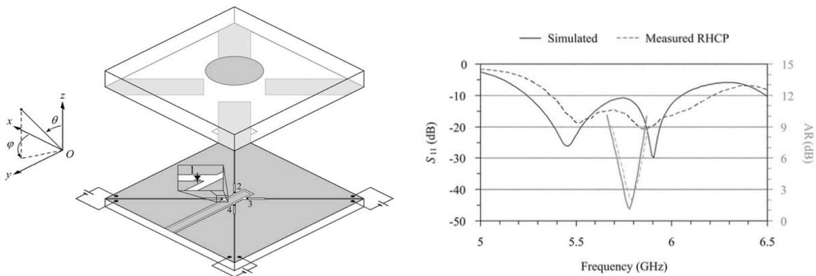
Figure 4.4: Circularly polarized reconfigurable structure and its results [7].
