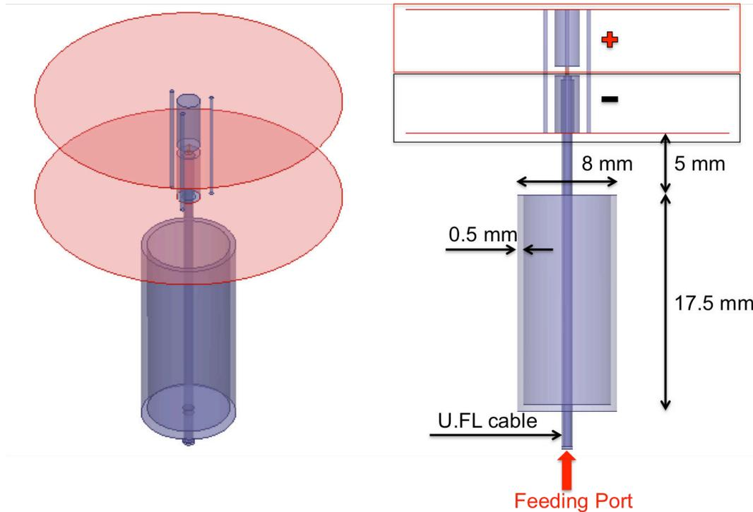
Figure 4.17: The balun structure integrated in the antenna.
