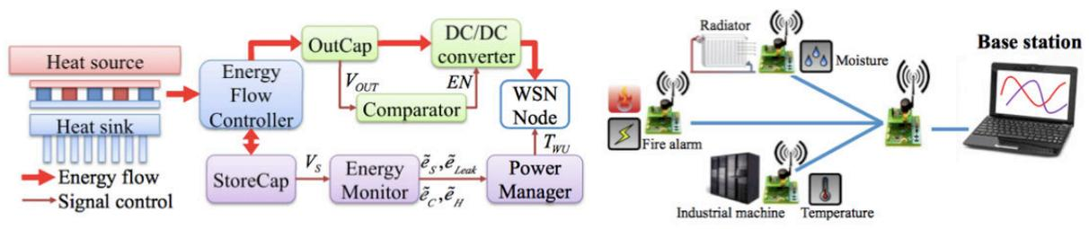
Figure 4.1: Generic architecture of the thermal-powered WSN node [1]
