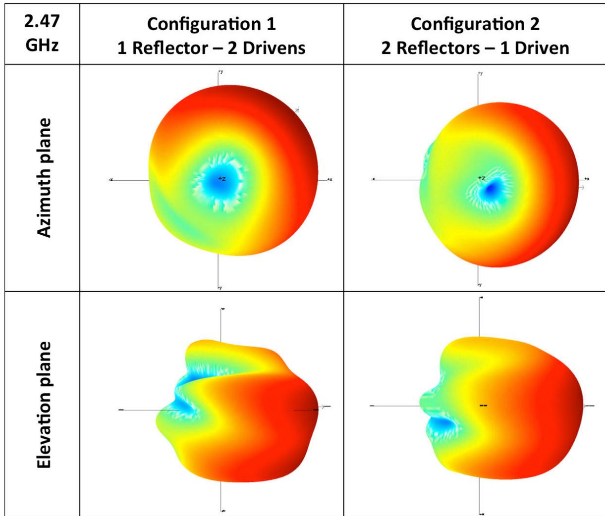
Figure 4.20: Measured 3D realized gain at 2.47 GHz
