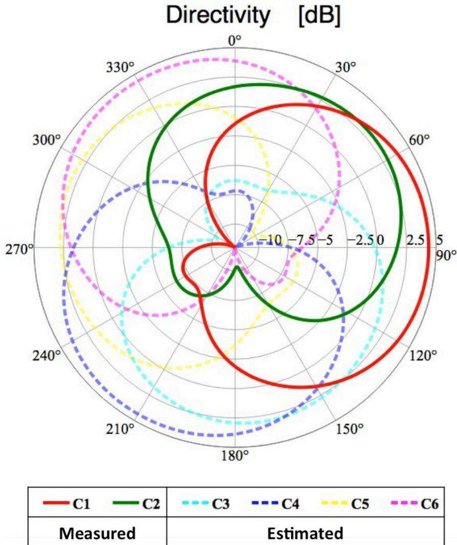
Figure 4.21: Estimated full configuration of the proposed antenna
