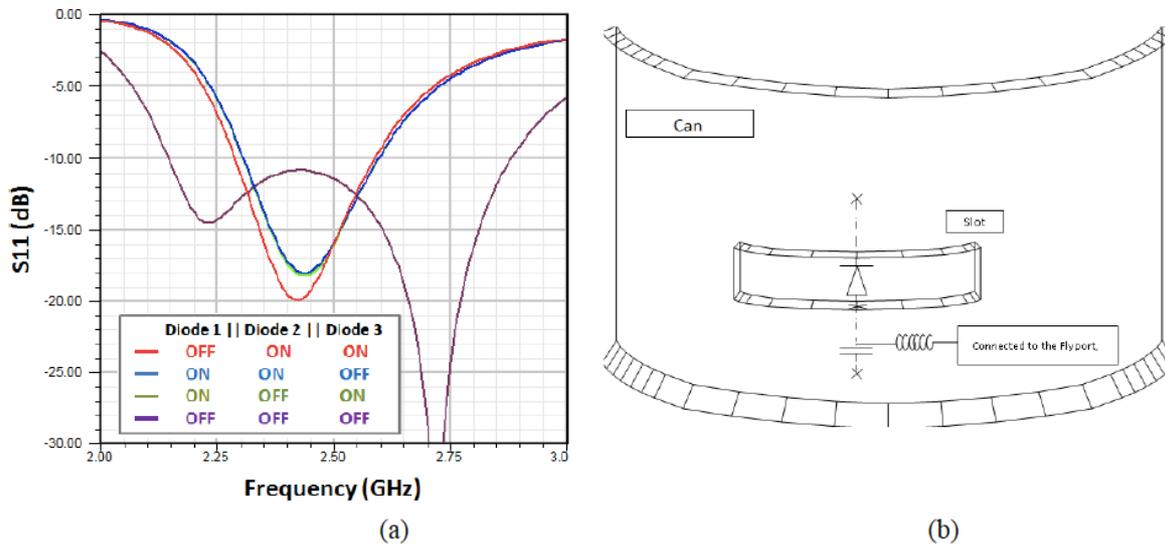
Figure 4.24: Simulated reflection coefficient and switch system topology.
