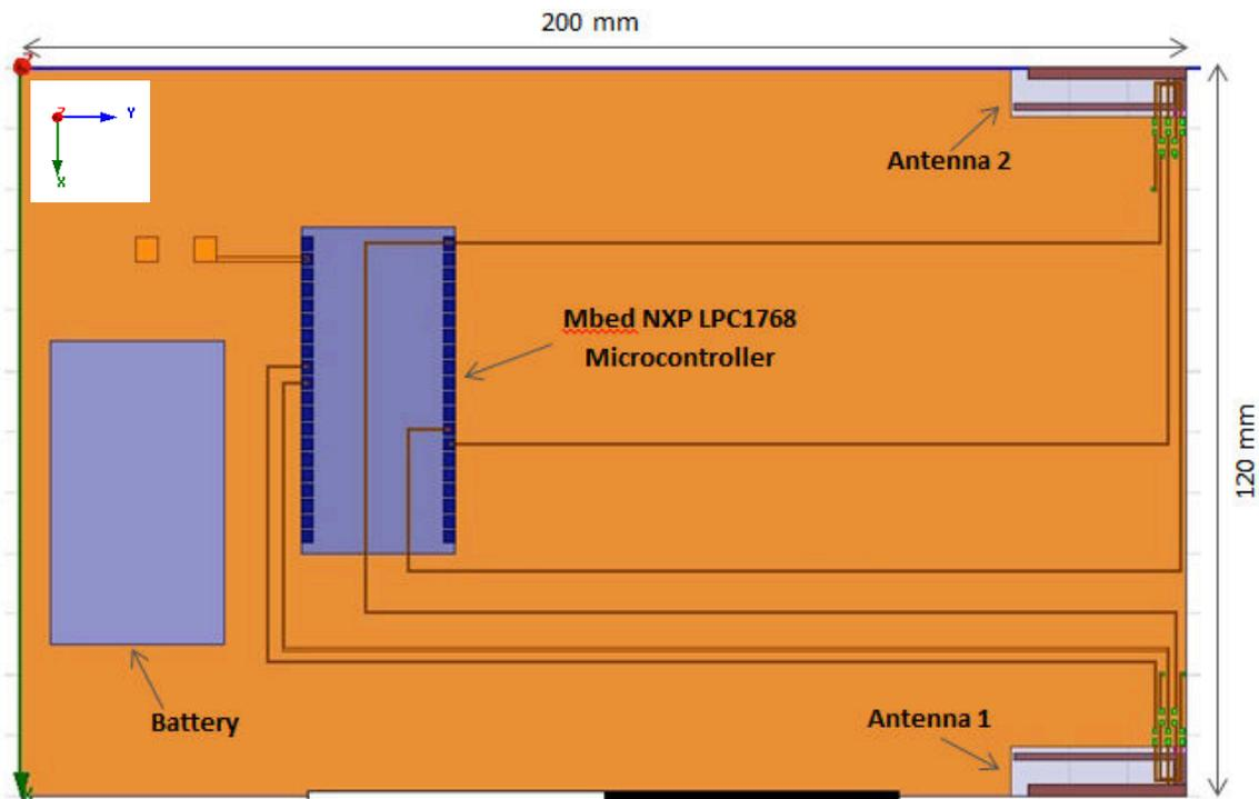
Figure 2.9: Top view of the reconfigurable antenna
