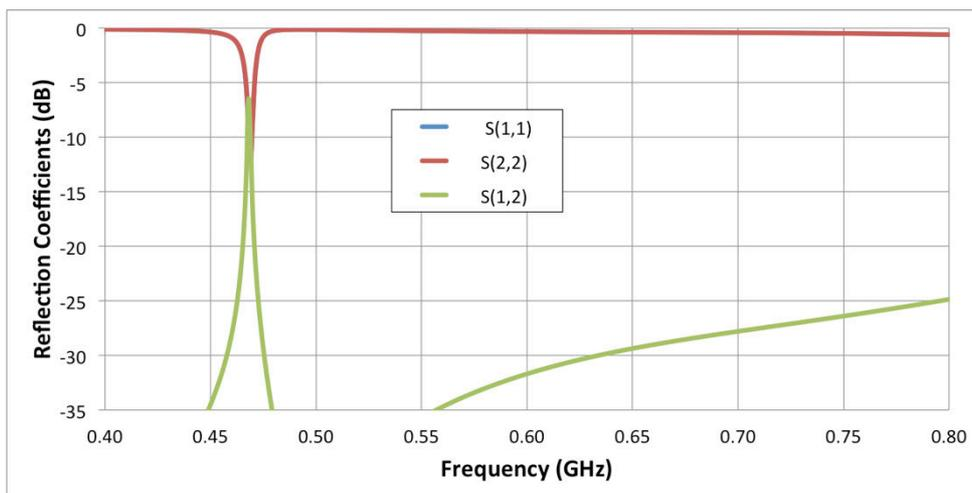
Figure 2.15: Config 3 - the resonances of antenna 1 at 470 MHz and antenna 2 at 470 MHz (The S11 and S22 results overlap each other)
