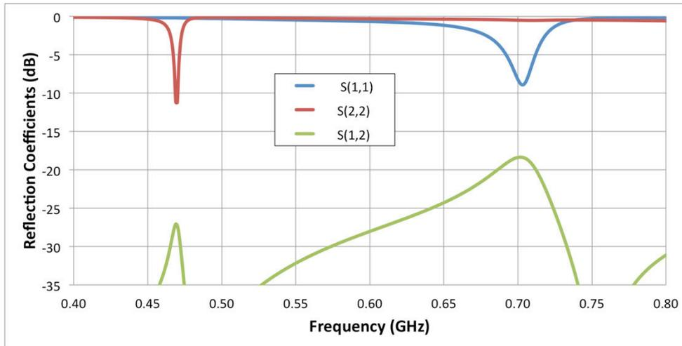
Figure 2.13: Config 2 - the resonances of antenna 1 at 700 MHz and antenna 2 at 470 MHz
