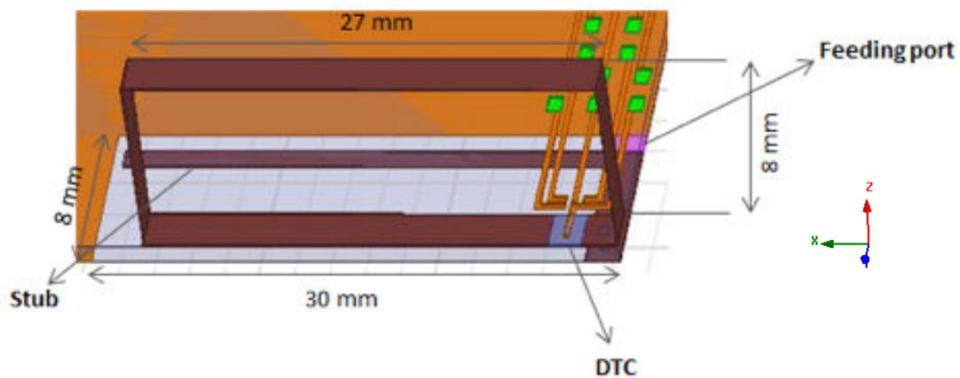
Figure 2.8: Antenna geometry
