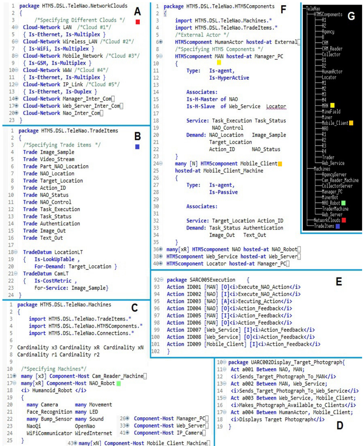
Figure 4.4: Excerpt of code written in HTM5-DSL for 'Teleroobotics On Nao' System. Section 'A': Cloud networks, Section 'B': Trade Information, Section 'C': Machines, Sections 'D' and 'E': Behavioural Elements and Section 'F': HTM5 Components. The code is executed to generate Java Class components (Model-to-Text) and UML class model (Model-to-Model). Section 'G' is the component directory structure generated as a result of code execution.
