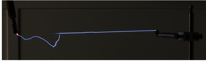
Figure 8.7: Photograph of a partially-guided discharge recorded with a 32 cm gap.
