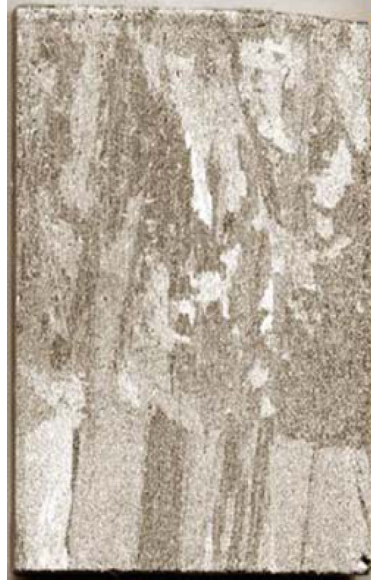
Figure 1.12: Picture that shows breakdown of the solidification front in MC Si [6].
