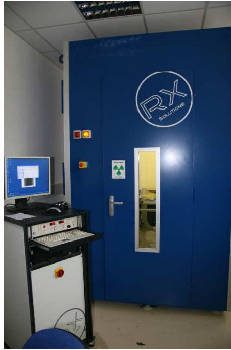
Figure 4.1: X-ray CT scanner at Laboratoire 3S-R
