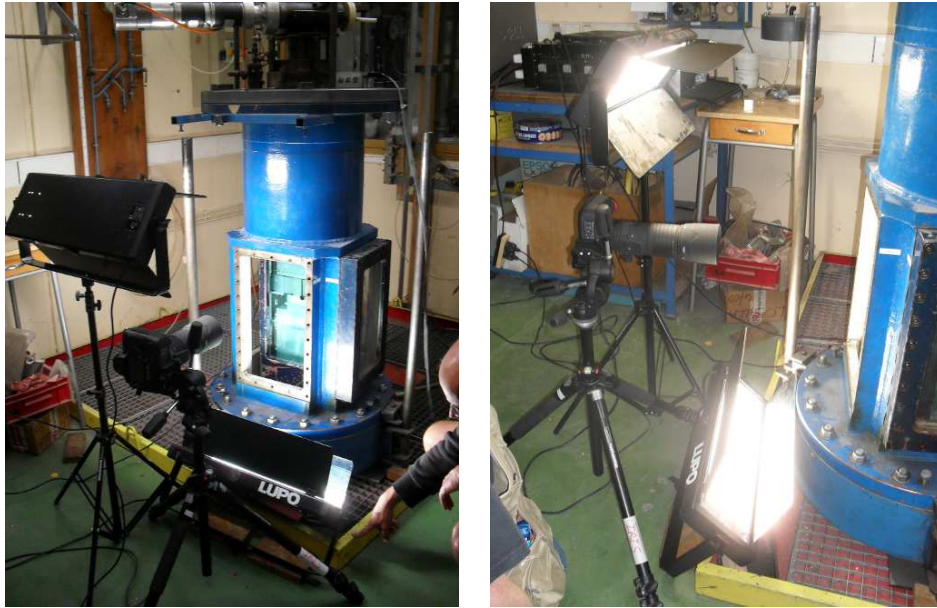
Figure 4.4: Experimental set up used to take pictures of the sample during the loading including the lighting and camera required to take the photographs used to carry out 2D-DIC.
