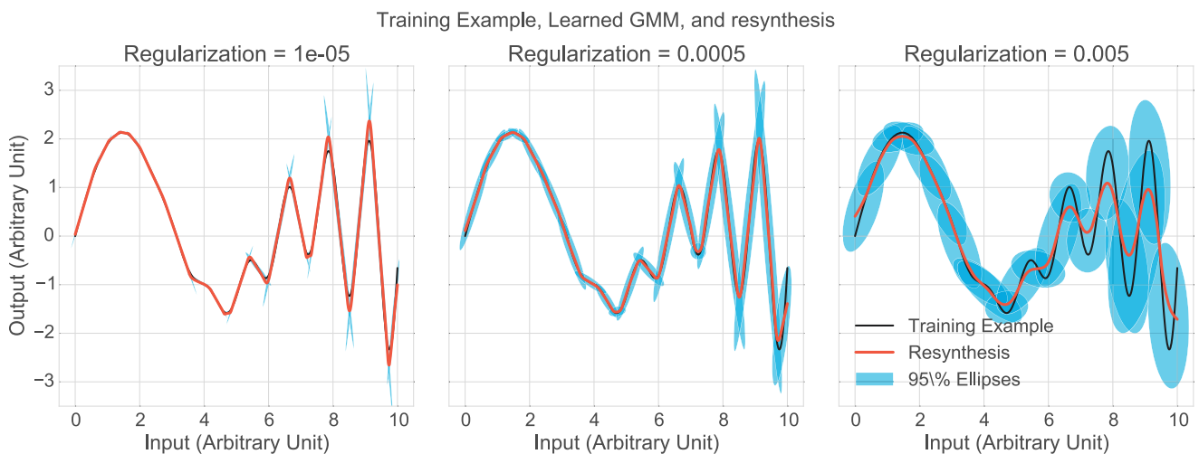
Figure 6.3: Example of Multimodal GMM and Gaussian Mixture Regression on artificial data. Various levels of regularization are used for comparison. The models were trained with 20 Gaussian Components.
