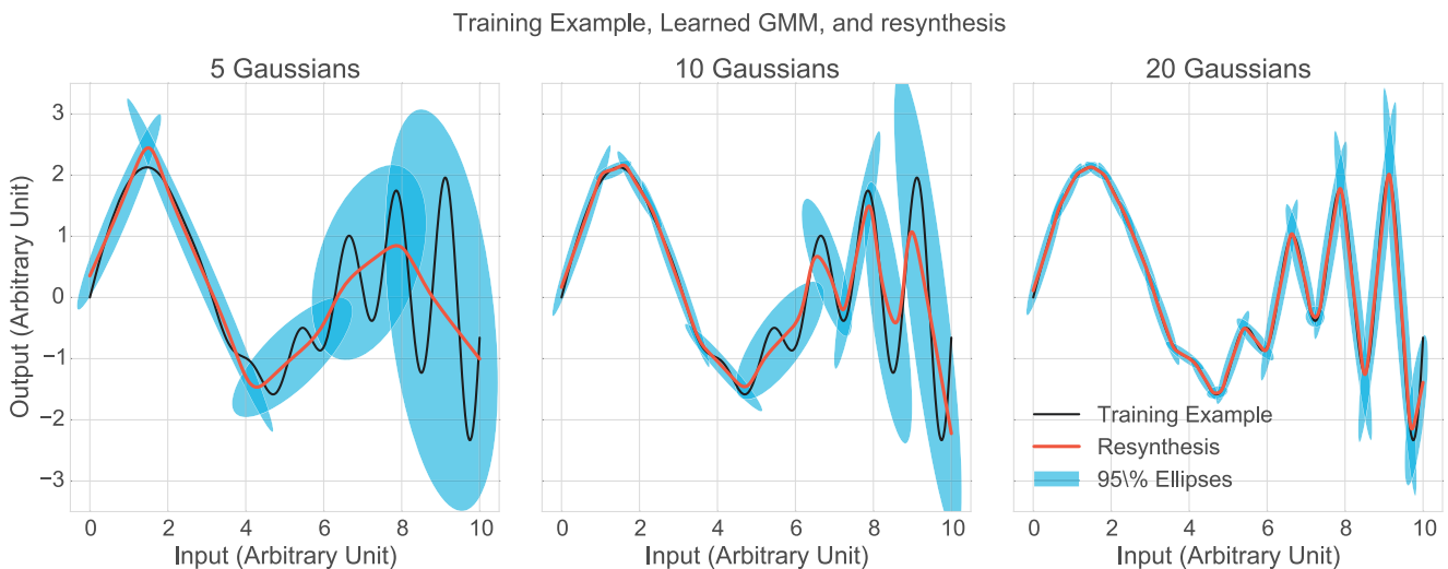
Figure 6.2: Example of Multimodal GMM and Gaussian Mixture Regression on artificial data. 5, 10 and 20 components are respectively used for comparison. The models were trained with regularization [\sigma] = 5e - 4
