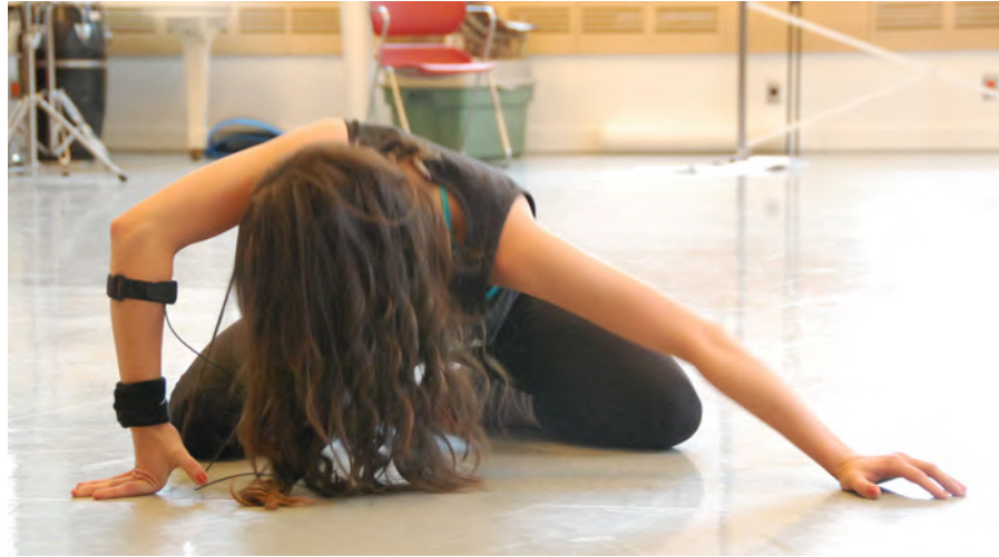
Figure 9.13: A participant equipped with the sensors: 3D accelerometer (wrist) and EMG (forearm).
