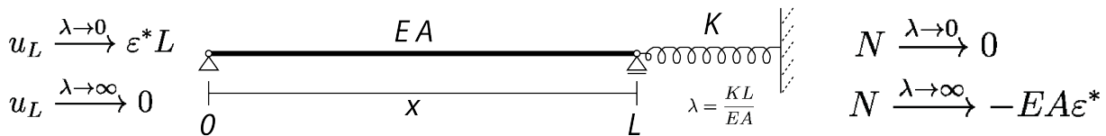
Figure 3.3 – One-dimensional bar of length L and stretching rigidity EA expanding against a spring of rigidity K . Depending on the rigidity contrast between the bar and the spring ( \lambda = KL/EA ), the eigenstrain is either converted into stress ( nilpotent ) or strain ( impotent ).
