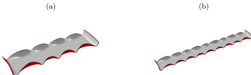
Figure 8.7 – Finite-element calculation also predicts tubular-wrinkling in the case of rectangular bilayers.
