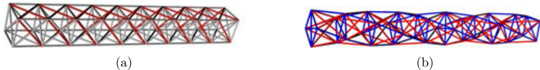
Figure 7.14 – Twisting corresponds to a different rest length of the diagonal springs spanning the sides of the extruded square lattice structure that represents a twister . (Left) Initial straight state with one set of diagonals activated. (Right) Final twisted state where the stress state redistributes across the springs. (Red) compression. (Blue) tension.
