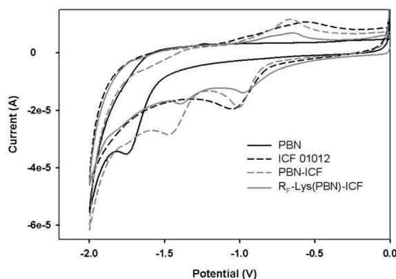
**Figure 3.2.5.** Reduction of PBN, ICF01012, PBN-ICF and R<sub>F</sub>-Lys(PBN)-ICF in 50 mM NaCl at 0.1 V/s.
