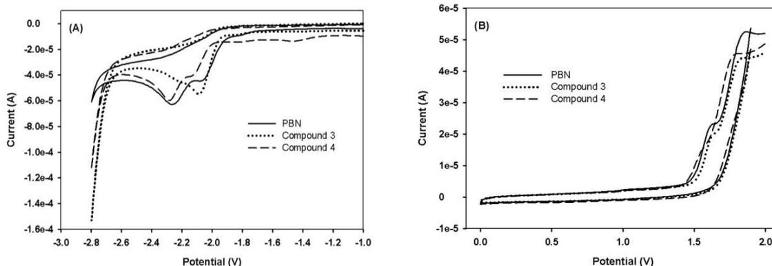
**Figure 2.3.3.** Cyclic voltammograms of PBN and compounds **3** and **4** in acetonitrile containing 50 mM of TBAP with a sweep rate of  $0.1 \text{ V}\cdot\text{s}^{-1}$ ; (A) reduction and (B) oxidation.
