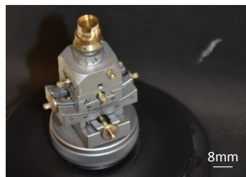
Figure 3.9 – Picture of the oriented 4-mm radius \text{TiO}_2 cylinder with the y -axis as the rotation axis.
