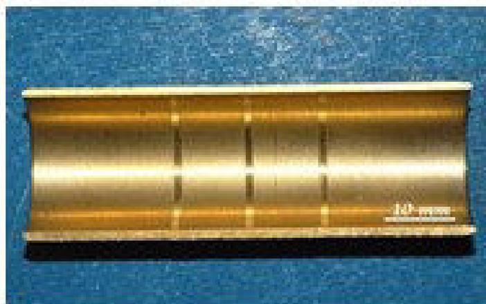
**Figure 3-16:** Longitudinal view of Al brass stepped specimens.
