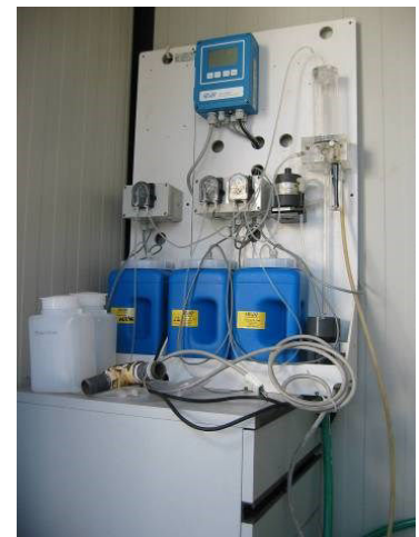
Figure 3-8: BIOX and chlorination treatments: (a) BIOX signal trend and residual oxidant concentration in seawater measured with the on-line instrumentation based on DPD colorimetric method, (b) AMI Codes (SWAN) colorimetric device.
