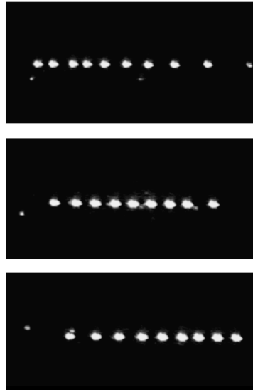
Fig. 4.15 Observation of a breathing mode: the displacement of the chain as a whole from the center with the inter-particles spacing increasing as one goes farther from the center of the array [38].
