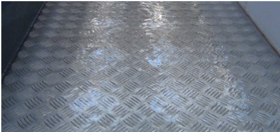
Figure 3.18: The channel with the aluminium roughness bottom
