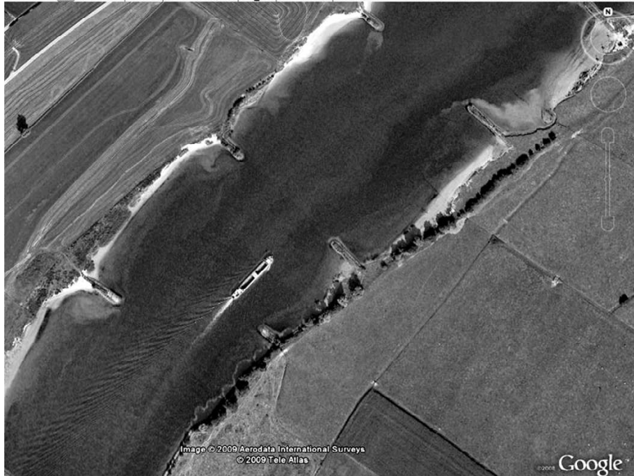
Figure 1.2: Separating and recirculating flow in groyne fields along the river. [Talstra, 2011]
