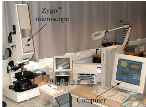
Fig III-3: Real view of ZYGO™ 200 interferometer microscope
