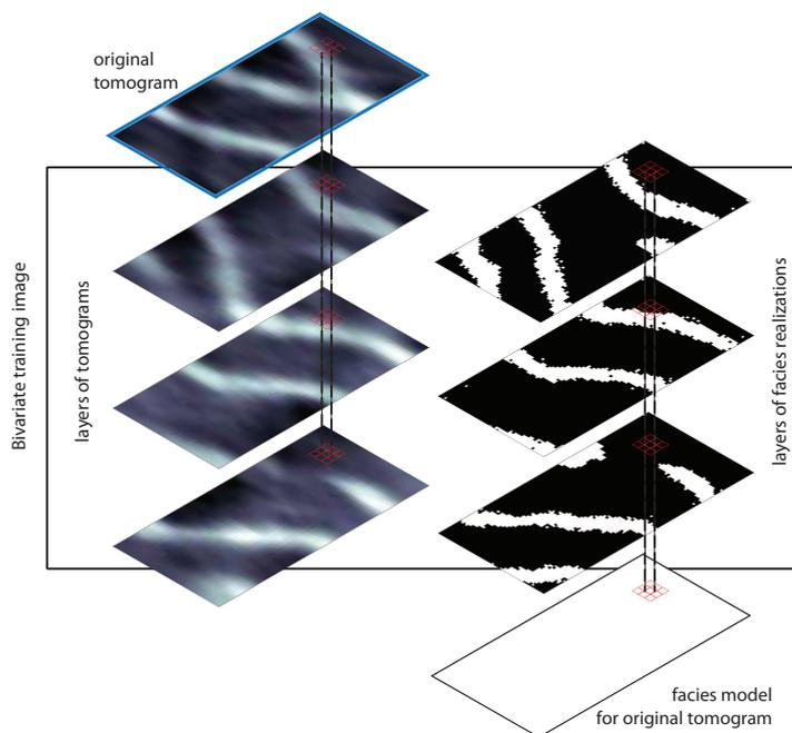
**Figure B.2:** The sampling principle used to account for the spatially variable resolution of geophysical tomograms.
