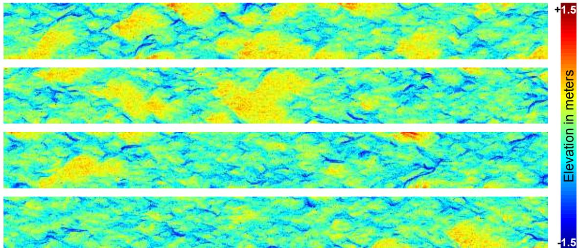
**Figure 3.3:**  $11600\text{ m} \times 1200\text{ m}$  ( $580\text{ pixels} \times 60\text{ pixels}$ ) simulations of DEMs with DS, using a monivariate TI. Red: highest elevations; blue: lowest elevations.
