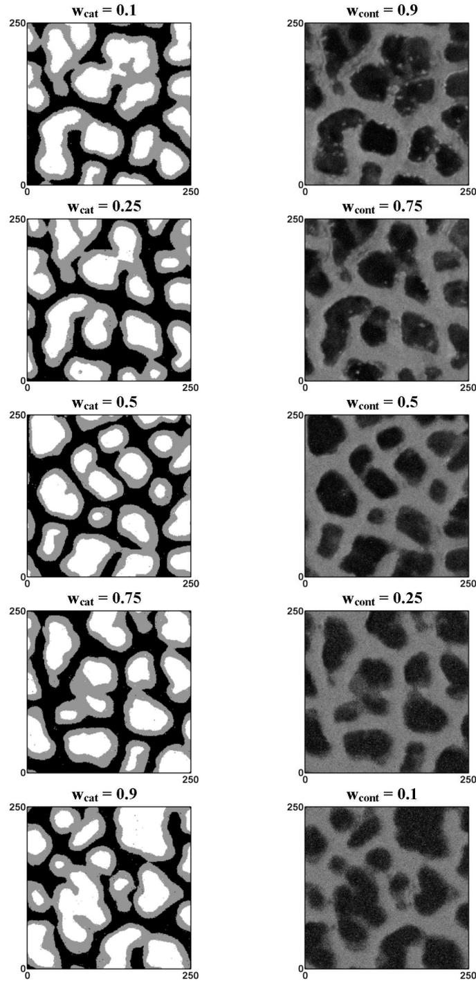
**Figure 2.12:** Illustration of the multivariate simulation option: five unconditional bivariate simulations using Fig. 2.1a and 2.1b as bivariate TI, and sensitivity analysis for the weights given to the two variables ( $w_{cat}$  and  $w_{cont}$ ). The left column represents the categorical variable for each simulation, and the right column represents the corresponding continuous variable.
