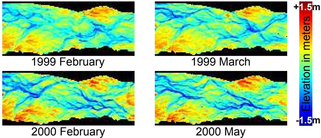
**Figure 3.2:**  $2900\text{ m} \times 1200\text{ m}$  ( $145\text{ pixels} \times 60\text{ pixels}$  -  $x$  axis  $\times$   $y$  axis) DEMs of the Waimakariri River, New Zealand at four time steps. Red: highest elevations; blue: lowest elevations.
