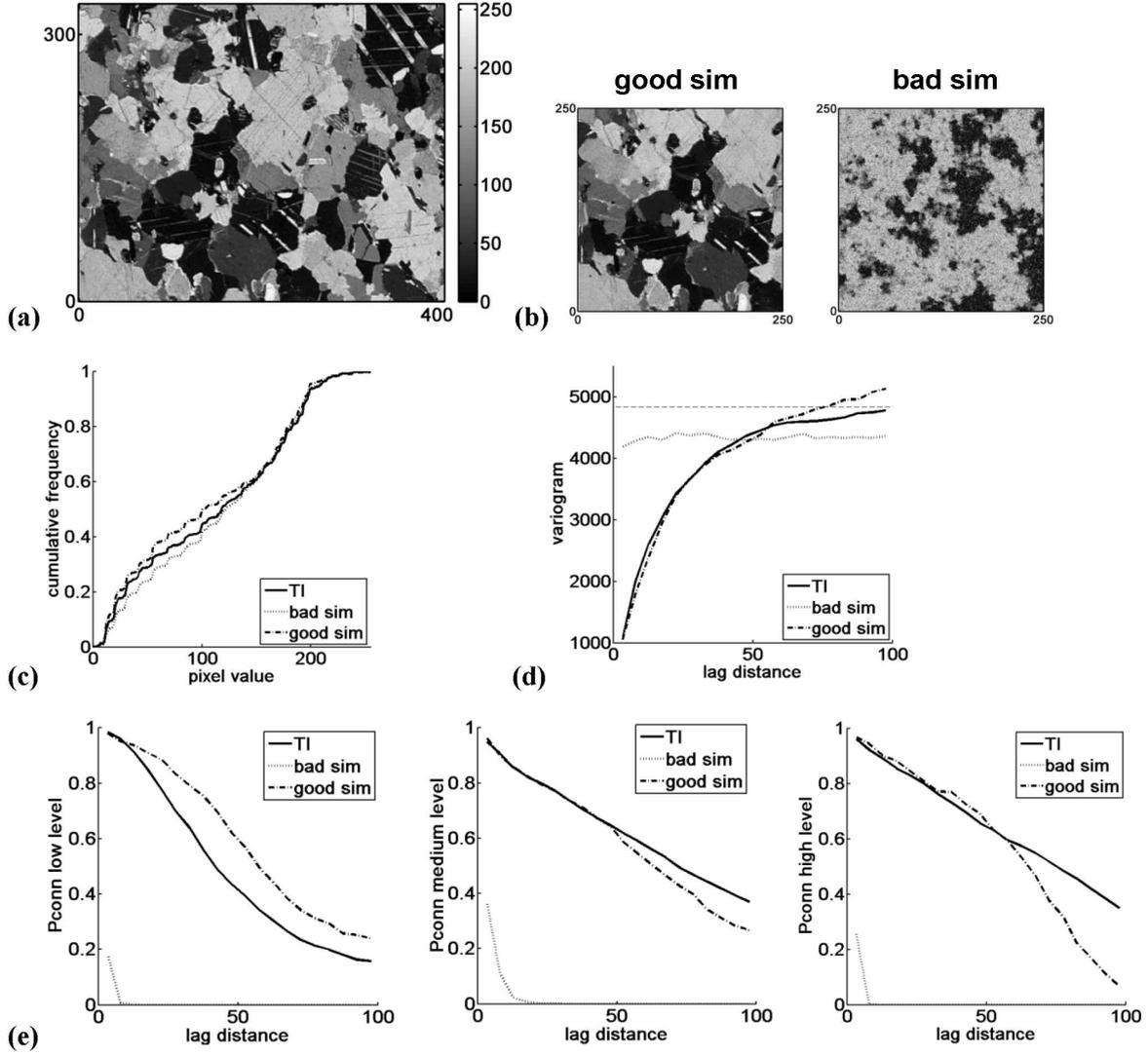
**Figure 2.7:** Reproduction of (a) the continuous marble TI statistics of (b) a good ( $t = 0.01$ ,  $f = 0.5$ ,  $n = 80$ ) and a bad simulation ( $t = 0.2$ ,  $f = 0.5$ ,  $n = 5$ ) with the reproduction of (c) the histogram, (d) the variogram (the dotted line represents the TI variance) and (e) the connectivity functions.
