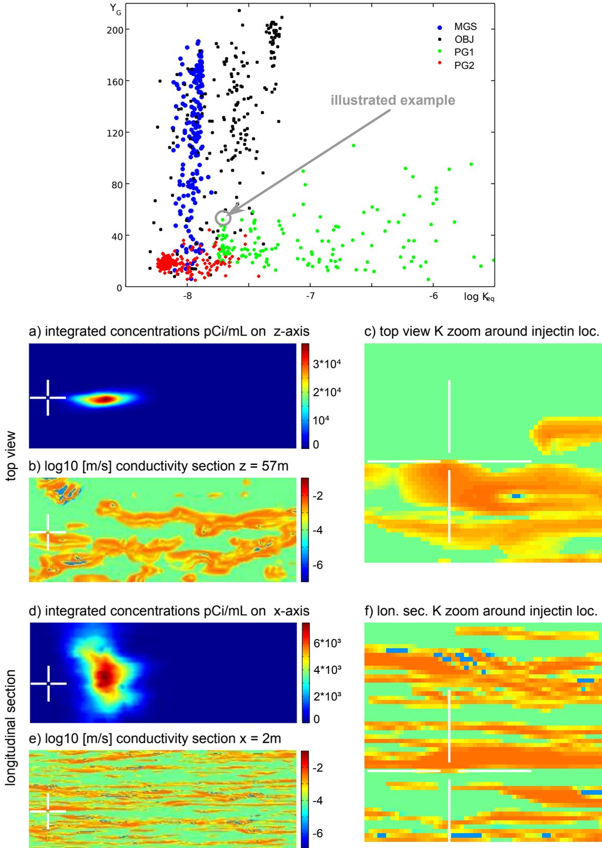
**Figure D.4:** Illustration of cumulative concentrations 328 days after injection and conductivity sections for a PG1 K-field – characterized by a high equivalent conductivity – generating a slow plume; the white cross locates the highest concentration 27 days after injection.
