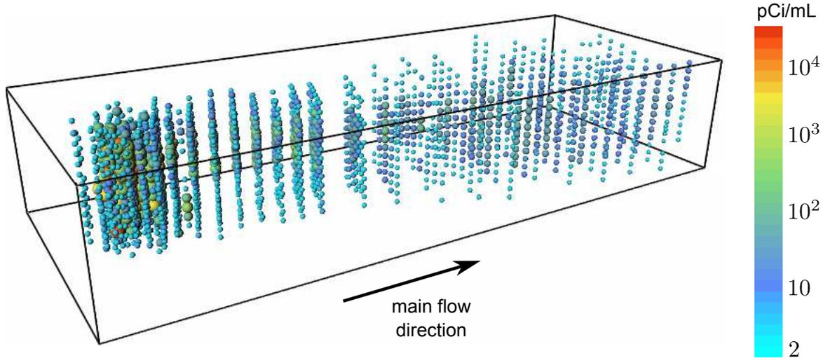
**Figure 5.2:** Reference concentrations measured 328 days after injection
