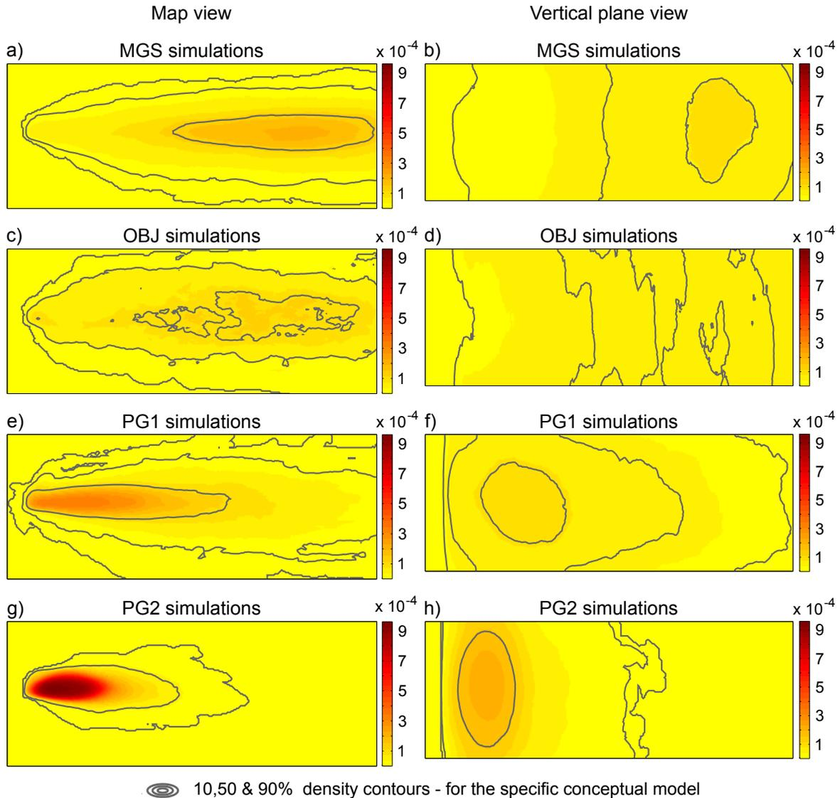
**Figure 5.12:** Probability densities per model for  $C \geq 16$  pCi/mL
