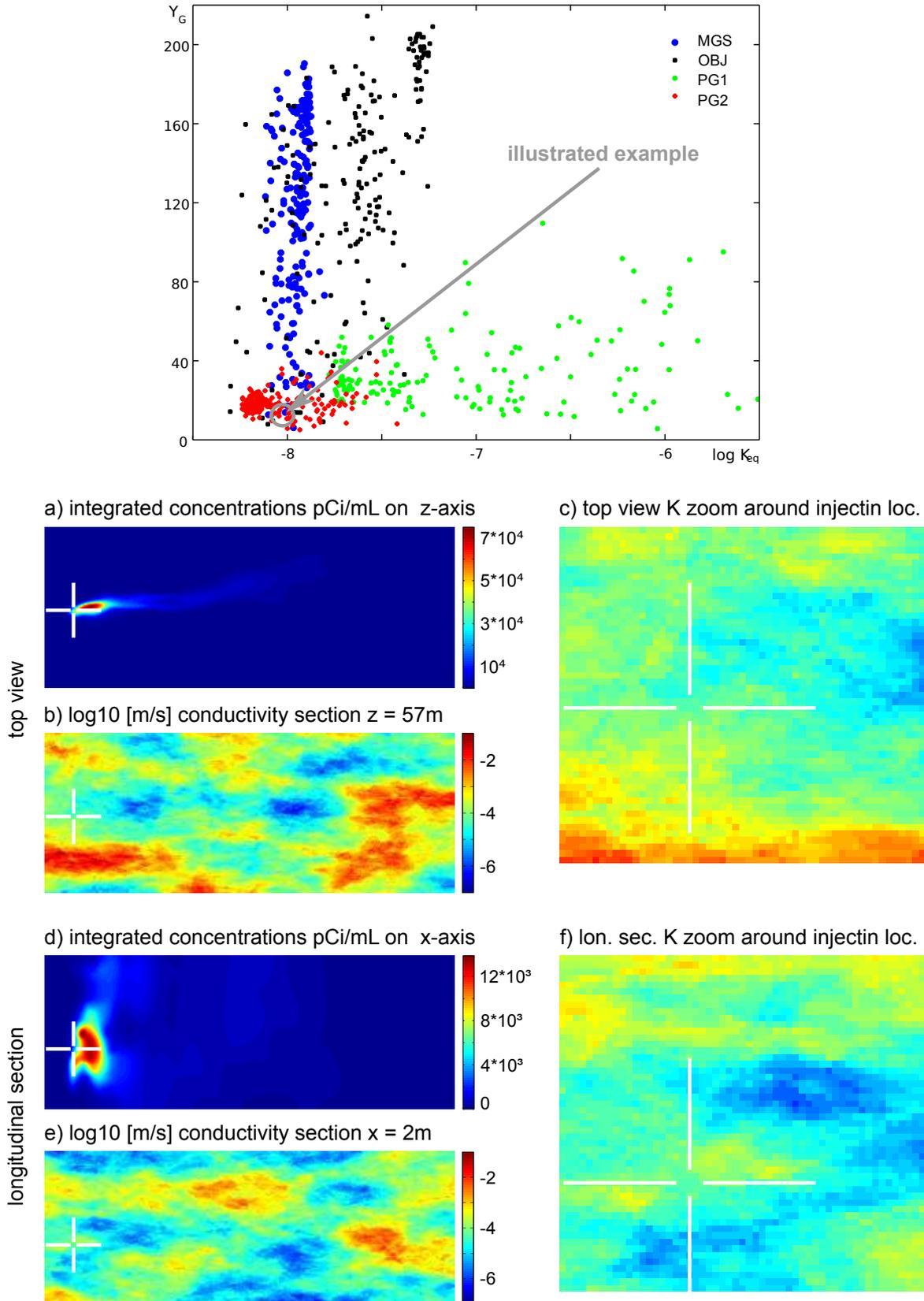
**Figure D.2:** Illustration of cumulative concentrations 328 days after injection and conductivity sections for a MGS K-field generating a slow plume; the white cross locates the highest concentration 27 days after injection.
