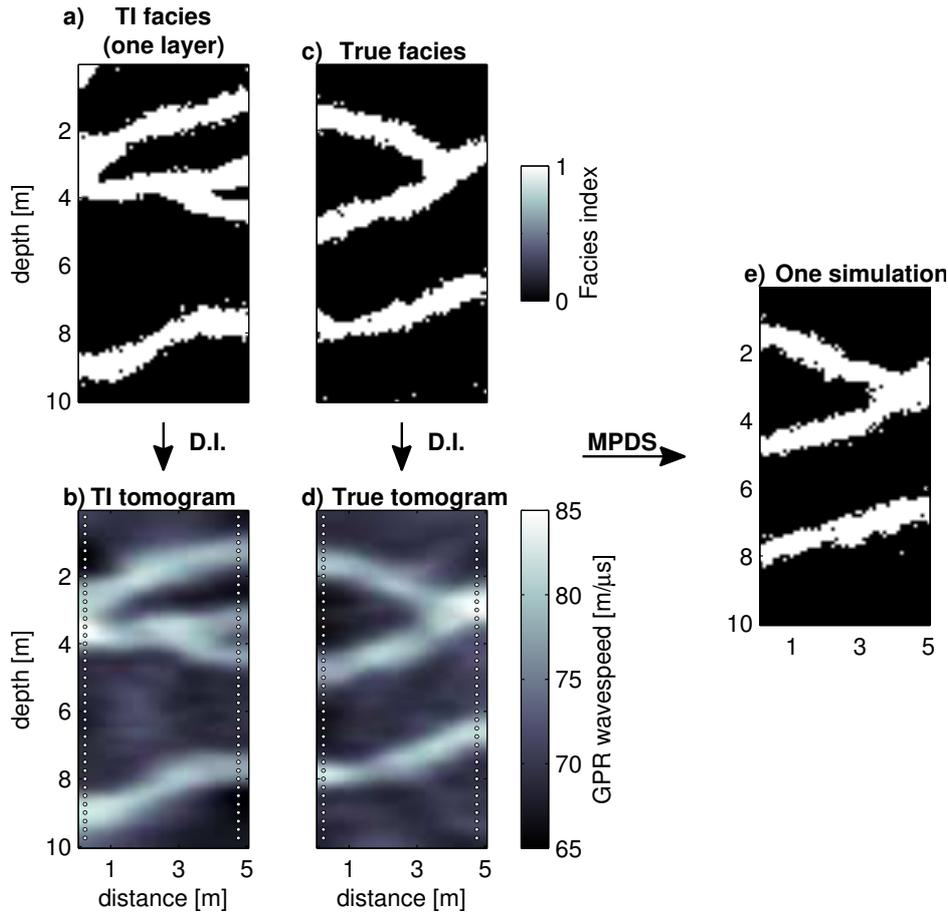
**Figure B.3:** (a) and (b): One layer of the bivariate training image; (a) facies and (b) corresponding tomogram. (c) The true facies we seek to recover and (d) its tomogram, which is used as conditioning data in the MPDS simulations. D.I. stands for deterministic inversion. White dots indicate transmitter and receiver positions for the radar traveltime calculations. (e) One simulated facies model.
