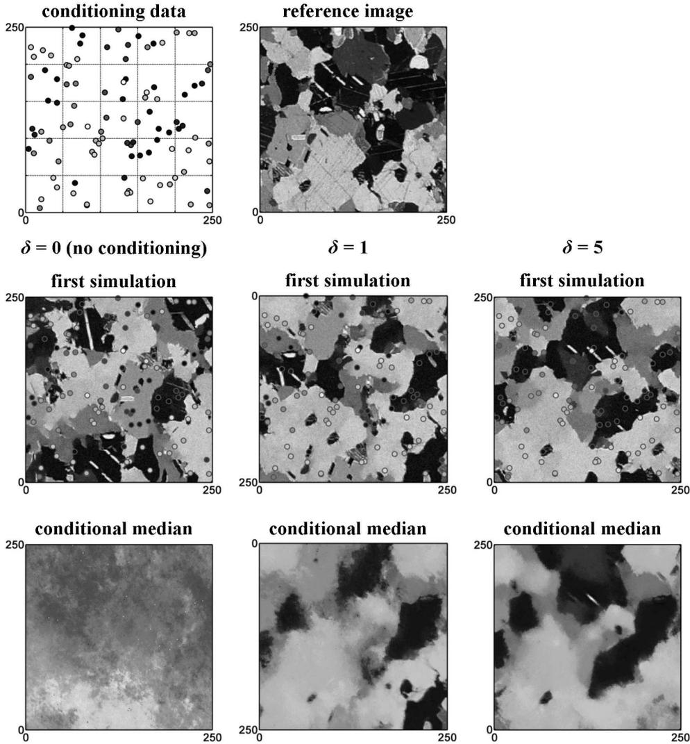
**Figure 2.14:** Illustration of data conditioning for the continuous marble TI (Fig. 2.1c) based on 100 conditioning data. For  $\delta = 0$ ,  $\delta = 1$  and  $\delta = 5$  the first simulation is shown together with the conditional median for each category summarizing 50 simulations.
