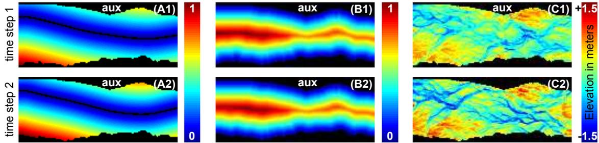
**Figure 3.8:** TI and its five auxiliary variables to simulate successive topographies: distance to centerline A1 at time step 1 and A2 at time step 2 ; distance to edges B1 at time step 1 and B2 at time step 2; elevation in meters C1 at time step 1 and C2 at time step 2.
