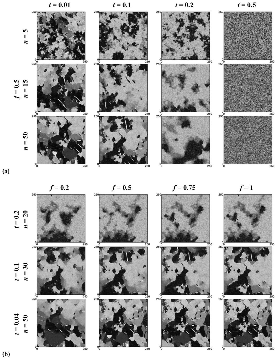
**Figure 2.5:** First out of 10 unconditional simulations illustrating the effect of parameters  $t$  and  $n$  with  $f = 0.5$  and (b) first out of 10 unconditional simulations illustrating the effect of  $f$  for constant  $t$  and  $n$  based on the continuous marble TI (Fig. 2.1c).
