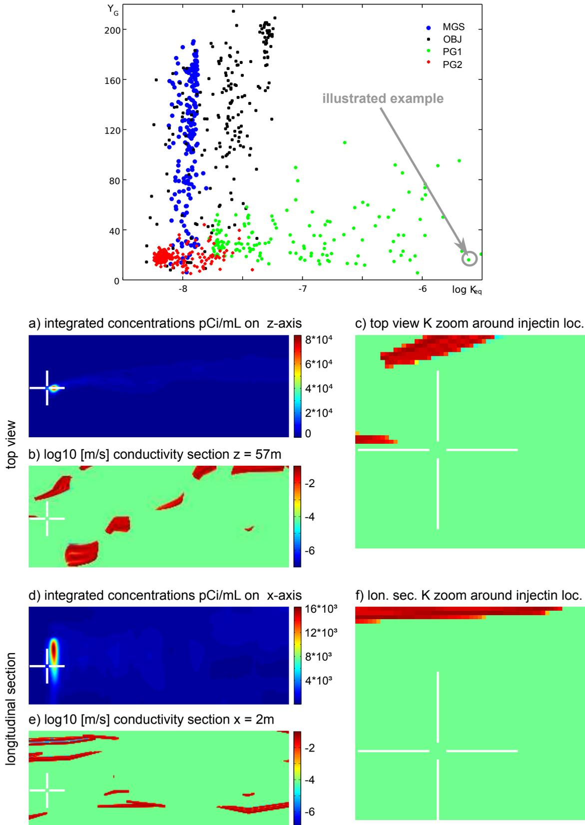
**Figure D.3:** Illustration of cumulative concentrations 328 days after injection and conductivity sections for a PG1 K-field – characterized by a low equivalent conductivity – generating a fast plume ; the white cross locates the highest concentration 27 days after injection.
