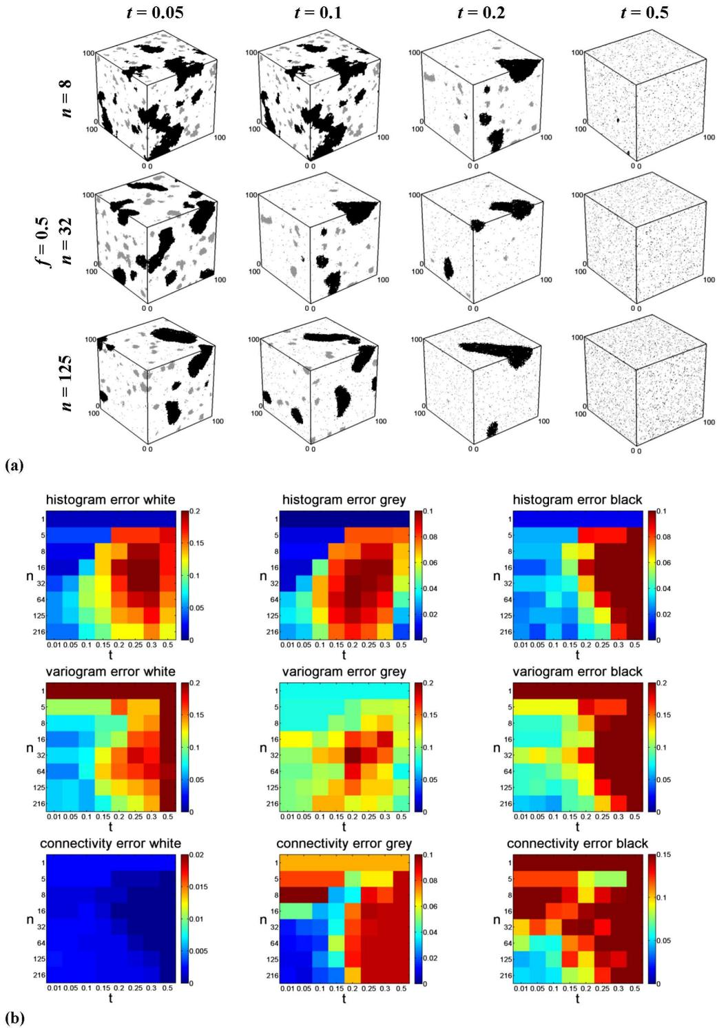
**Figure 2.10:** 3D example with (a) first out of 10 unconditional simulations illustrating the effect of parameters  $t$  and  $n$  with  $f = 0.5$  and (b) influence of  $t$  and  $n$  (for  $f = 0.5$ ) on the quality indicators based on the 3D concrete TI (Fig. 2.1g).
