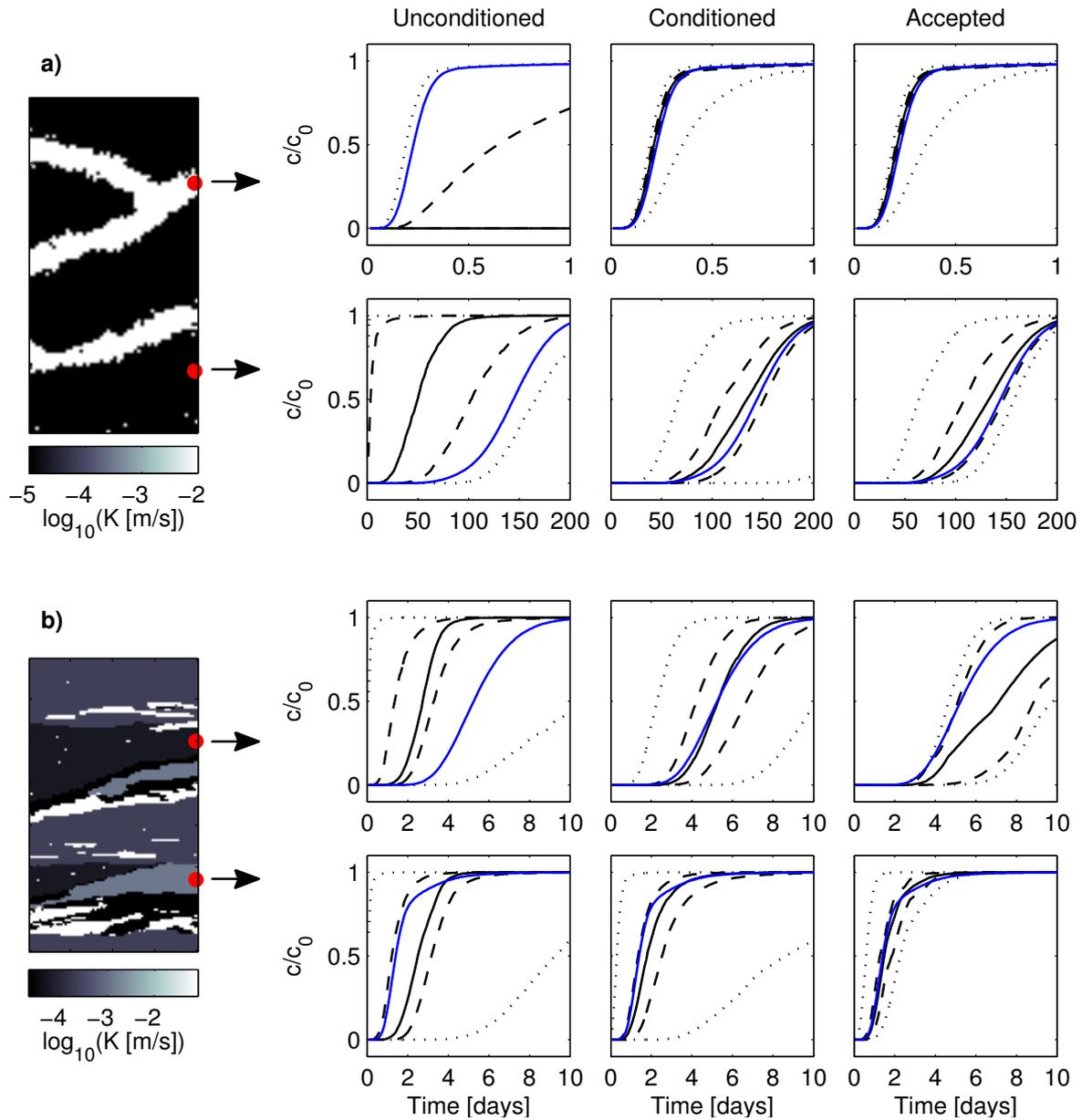
**Figure B.9:** Statistics of calculated breakthrough curves for (a) channel scenario and (b) Herten scenario. Solid, dashed and dotted lines depict mean, 50 % quantiles and 95 % quantiles. Blue line: breakthrough of the true model.
