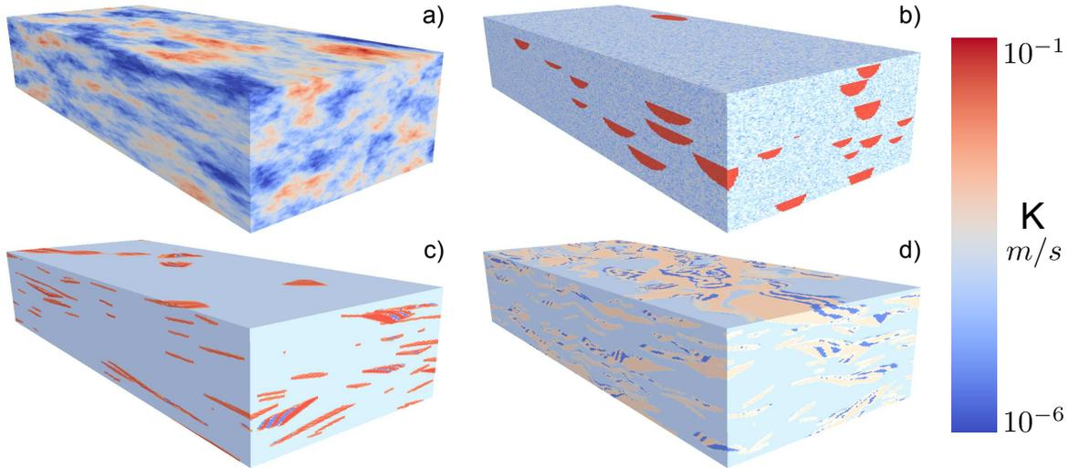
**Figure 5.4:** Three dimensional representations of scenario 3 conductivity fields for the different conceptual geological models (a): MGS, b): OBJ, c): PG1, d): PG2)
