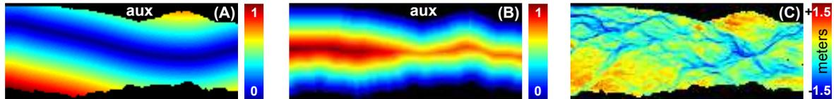
**Figure 3.6:** Auxiliary variables (A,B) and variable of interest (C) for the TI; (A) distance to centerline, (B) distance to edges, (C) topography.
