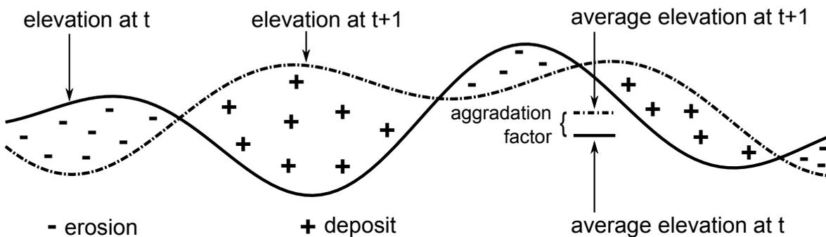
**Figure 4.2:** Pseudo processes of erosion and deposit
