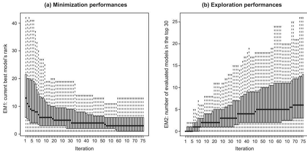
**Figure A.12:** Performances of the ProKSI algorithm (based on proxy 1) without power transform of the misfit. (a) box-plot of EM1 over the 100 replicates of the numerical experiment. (b) box-plot of EM2.
