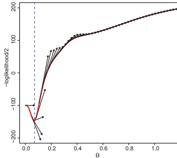
**Figure A.8:** Identification of  $\theta$  by maximizing the concentrated log-likelihood function. The large curvature at the minimum indicates a well-identified parameter value. The arrows stand for the gradients of the log-likelihood function, which have been calculated analytically, and are used within the optimization procedure.
