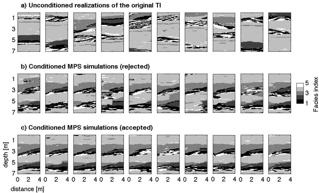
**Figure B.8:** Different MPDS simulations of the Herten training image in movie illustration. (a) Unconditioned simulations as they are used as layers of the training image. (b) MPDS simulations conditioned to a geophysical tomogram. These simulations failed to predict the radar data satisfactorily and were rejected. (c) As for (b) but with radar traveltimes for which the WRMSE is below the threshold, these simulation were accepted.
