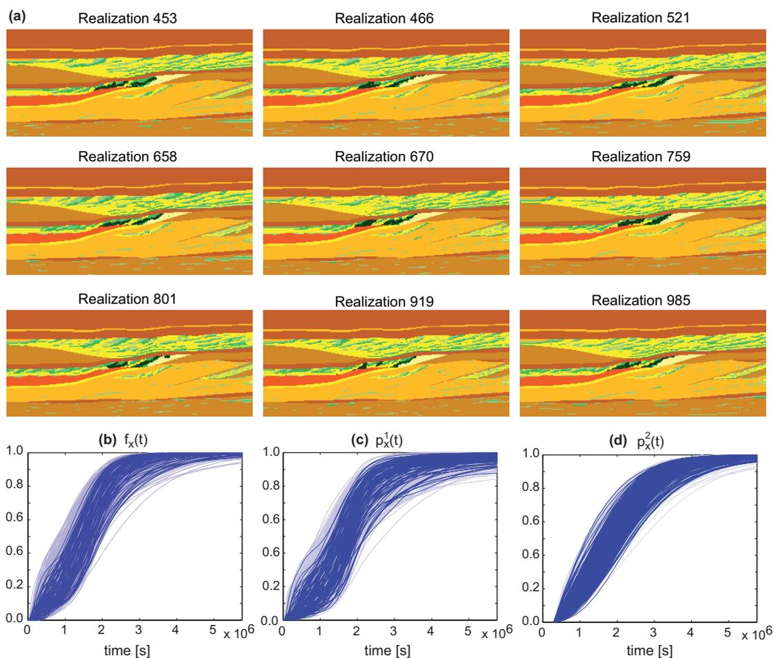
**Figure A.5:** (a) 9 realizations of the lithofacies. Because all the simulations are constrained by the large scale structure data, only the internal architecture within the main layers is displaying some variability between the simulations. (b) Ensemble of the breakthrough curves obtained with the accurate numerical model and the two proxies (c and d) for the 1000 parameter fields. To make the Fig. more readable, some breakthrough curves are represented in light gray color.
