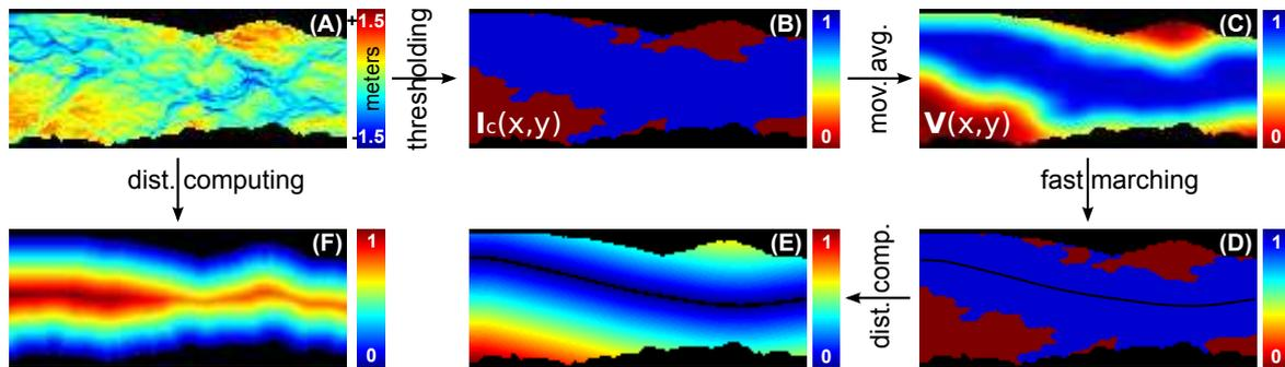
**Figure 3.4:** Auxiliary variables workflow. (A) initial DEM; (B) main channel; (C) velocity field; (D) main channel and its centerline; (E) normalized distance to the centerline; (F) normalized distance to the edges.
