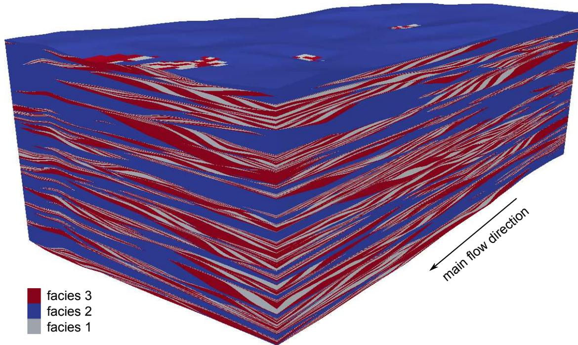
**Figure 4.7:** 3D heterogeneous facies model – example 3 – obtained with  $n = 10$  inner-layer iterative deformations, a flow power  $f_p = 5$  and an aggradation  $\alpha = 0.3 m$
