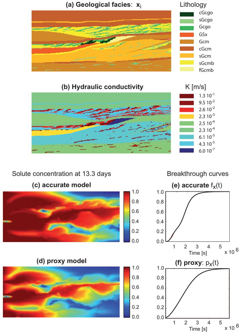
**Figure A.4:** Illustration of the main components of the illustrative example: (a) one simulation of a categorical field representing the geological facies. Each color corresponds to a type of sediment; (b) hydraulic conductivity field derived from the geological facies; (c,f) computation of the transient distribution of the concentration fields and breakthrough curve using an accurate numerical simulator; (d,f) approximation using a proxy simulator.
