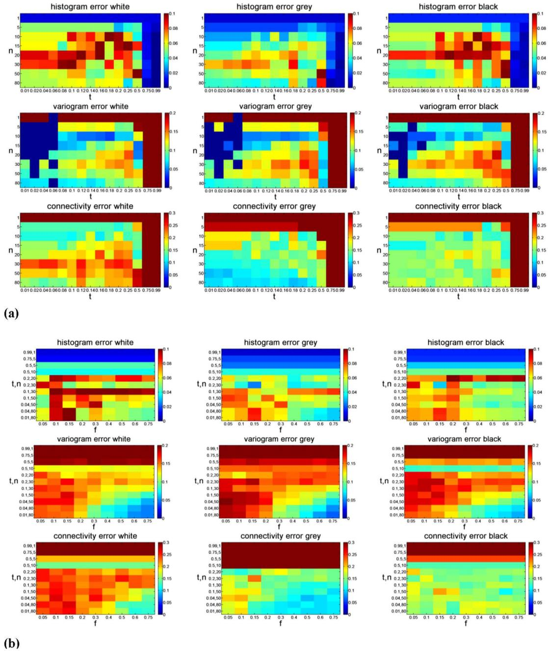
Figure C.6: Influence of (a)  $t$  and  $n$  (for  $f=0.5$ ) and (b)  $f$  on the quality indicators based on the categorical marble TI (Fig. 2.1d)
