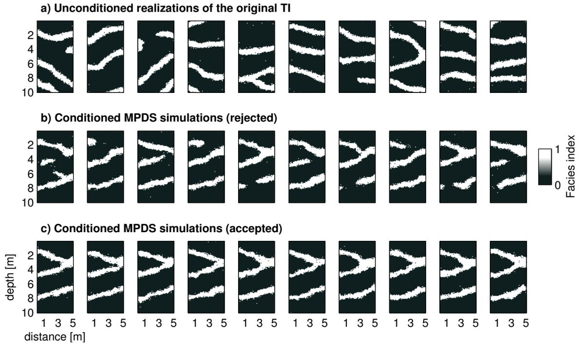
**Figure B.5:** Different MPDS simulations of the channel scenario in movie illustration. (a) Unconditioned simulations as they are used as layers of the ‘working training image’. (b) MPDS simulations conditioned to a geophysical tomogram. These simulations failed to predict the radar data satisfactorily and were rejected. (c) As for (b) but with radar traveltimes for which the WRMSE is below the threshold, these simulation were accepted.
