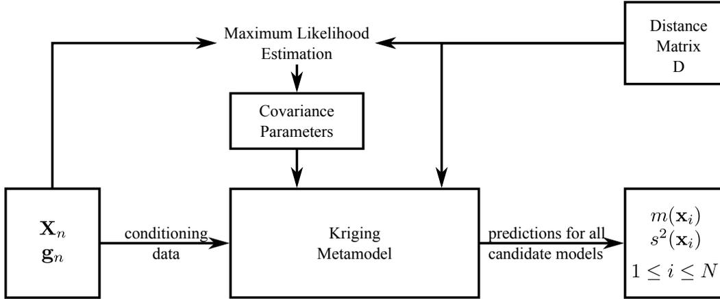
**Figure A.3:** Overview of the proxy-based kriging prediction workflow (after misfit transformation).
