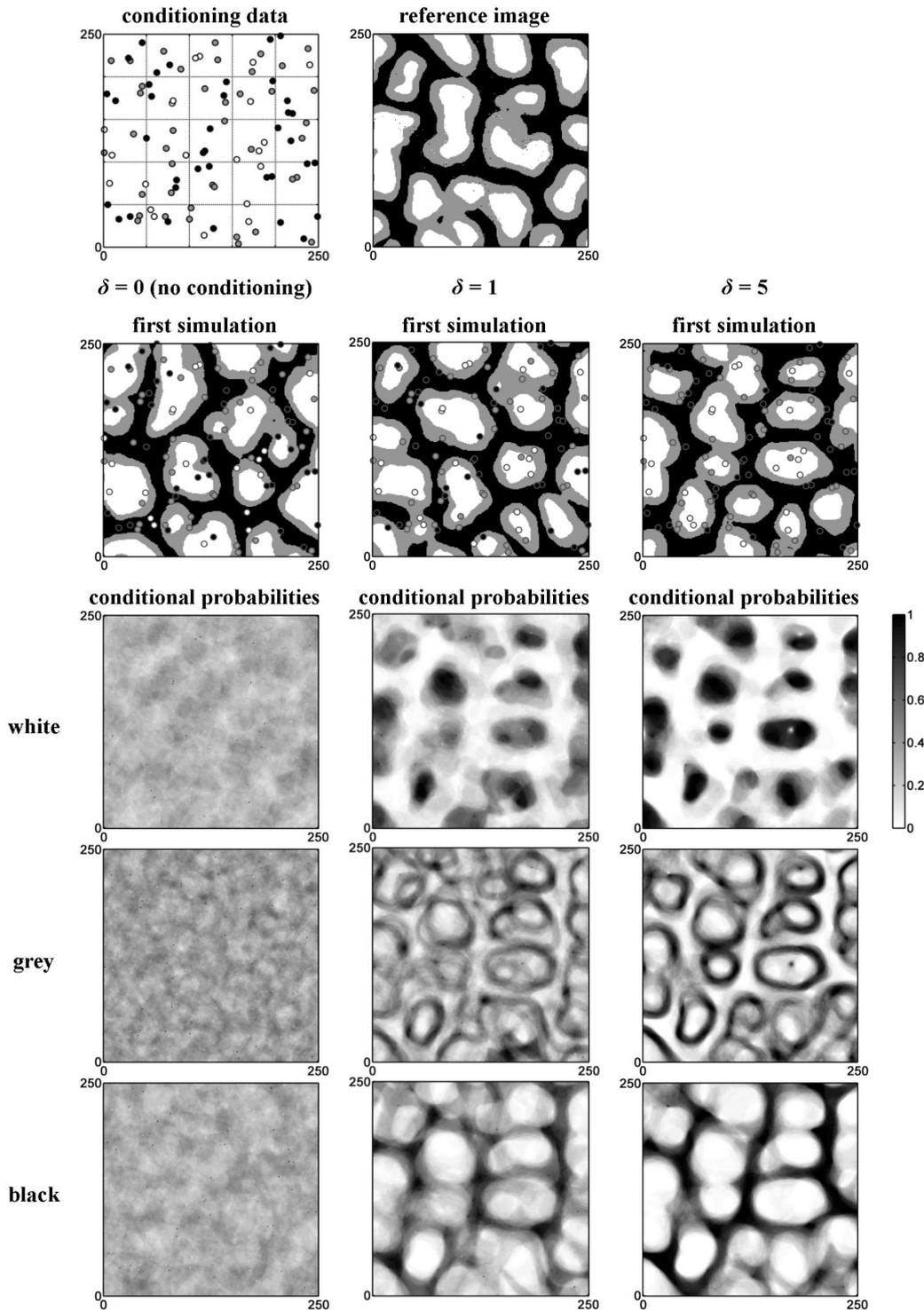
**Figure 2.13:** Illustration of data conditioning for the categorical ice-wedge TI (Fig. 2.1b) based on 100 conditioning data. For  $\delta = 0$ ,  $\delta = 1$  and  $\delta = 5$  the first simulation is shown together with the conditional probabilities for each category summarizing 50 simulations.
