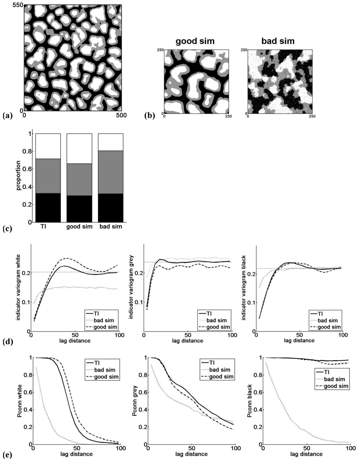
**Figure 2.6:** Reproduction of (a) the categorical ice-wedge TI statistics of (b) a good ( $t = 0.01$ ,  $f = 0.5$ ,  $n = 80$ ) and a bad simulation ( $t = 0.5$ ,  $f = 0.5$ ,  $n = 15$ ) with the reproduction of (c) the histogram, (d) the indicator variograms (the dotted lines represent the TI indicator variance) and (e) the connectivity functions.
