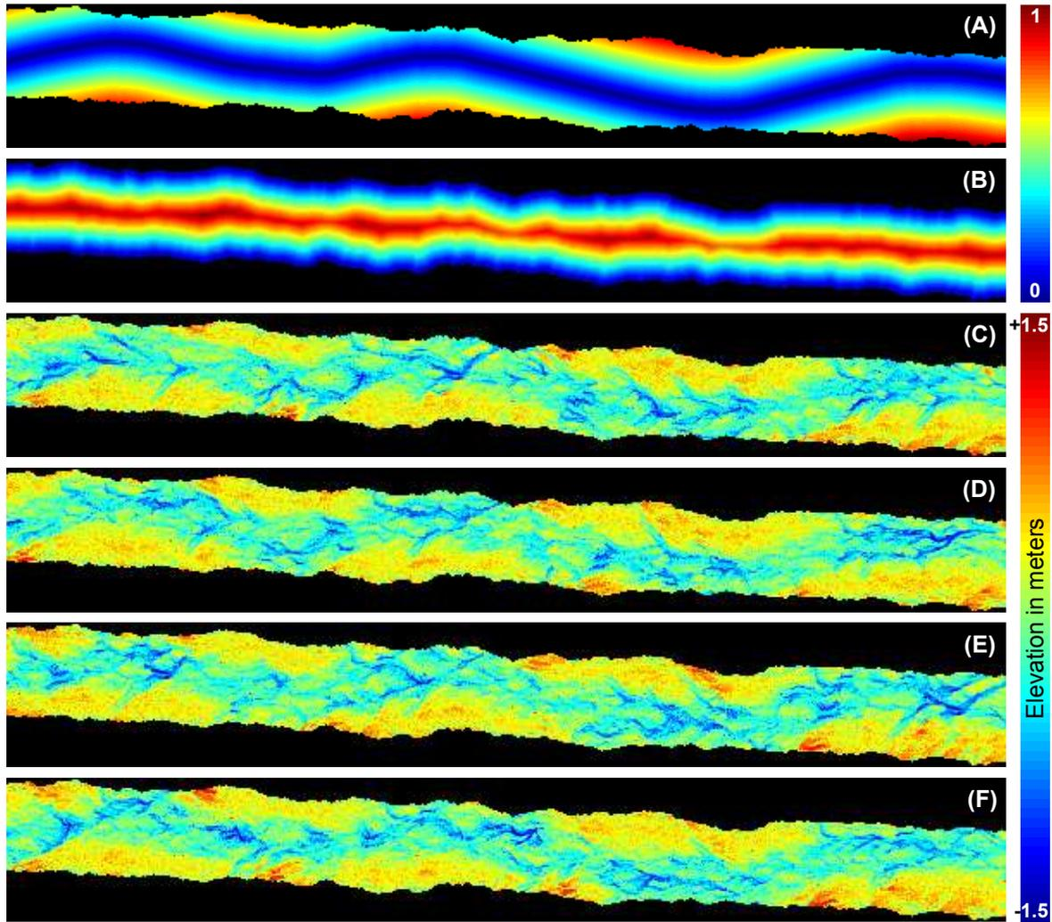
**Figure 3.7:** Conditioning data: (A) distance to the centerline, (B) distance to the edges, and four DEMs' simulations (C), (D), (E), and (F) with a three variables TI.
