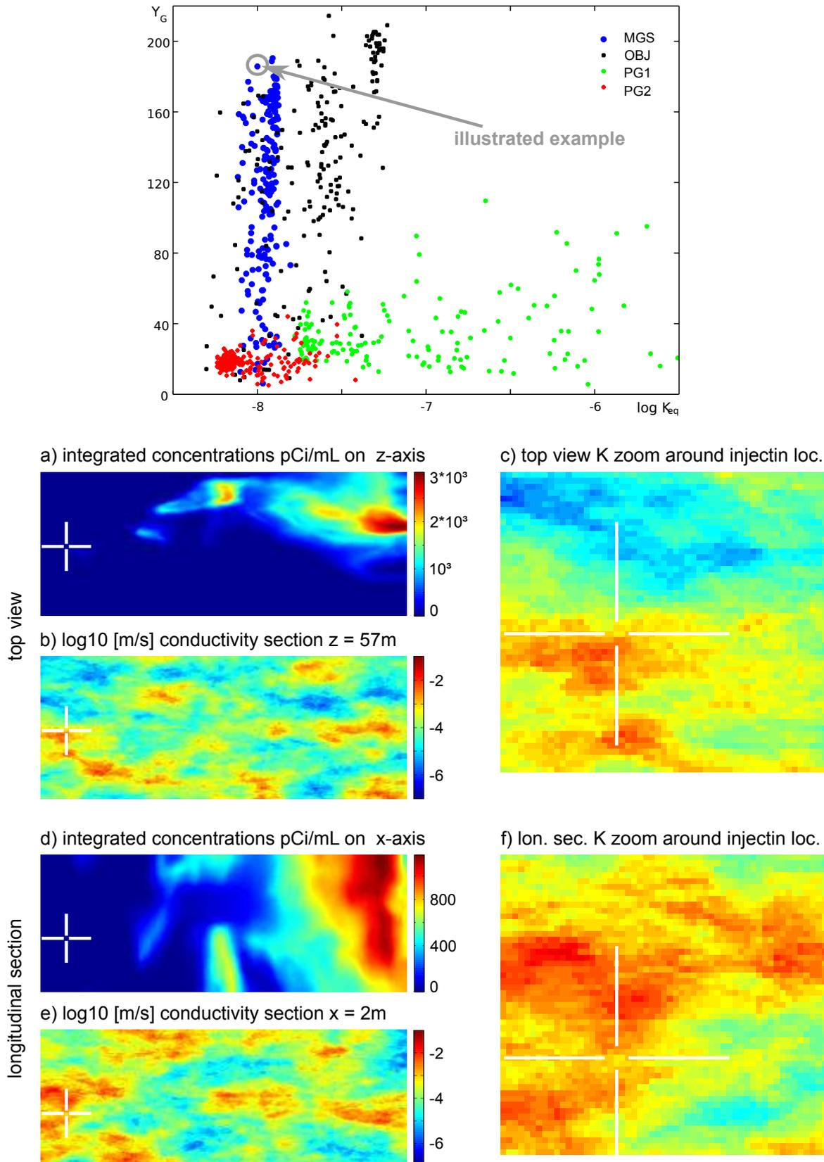
**Figure D.1:** Illustration of cumulative concentrations 328 days after injection and conductivity sections for a MGS K-field generating a fast plume; the white cross locates the highest concentration 27 days after injection.
