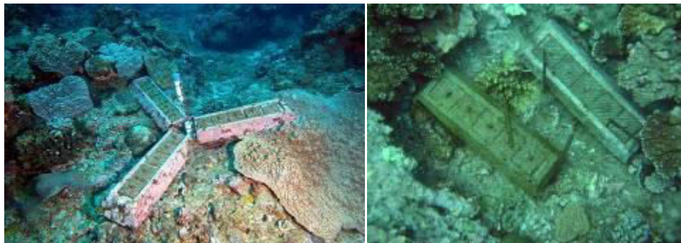
Figure 21: Cement structure used for the fixation of settlement tiles in the coral recruitment survey in A) South Africa and B) Reunion. Y-frame
