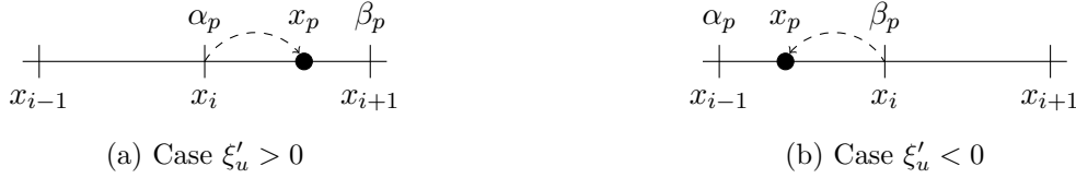
Figure VI.2: 1D configuration after a transport step in physical space (same behaviour in velocity space with \xi'_u \equiv a_u )
