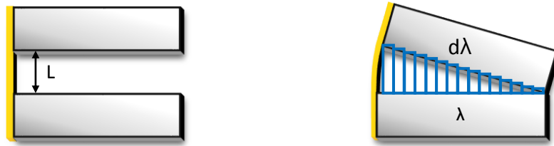
Figure 19: The Casimir force between a tweezer jaws is of the order of picoNewtons when they are parallel (left) or closed (right). In comparison, the magnetic force exerted on the upper jaw by an external magnetic field can reach 140 nN.
