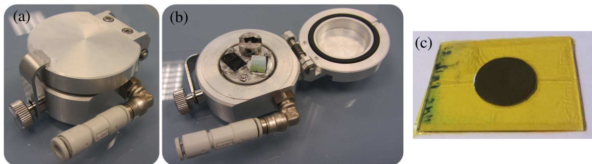
Figure 2-3. SEM transfer box permitting to keep the analyzed samples under argon protective atmosphere without air exposure at any step of the measurement (a,b); XRD sample protected by thin Kapton ® film (c).
