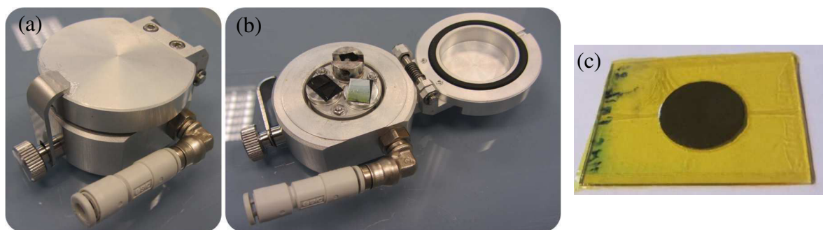
Figure 2-3. SEM transfer box permitting to keep the analyzed samples under argon protective atmosphere without air exposure at any step of the measurement (a,b); XRD sample protected by thin Kapton ® film (c).
