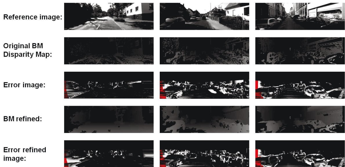
Figure 4.4 – Final result for the disparity map refinement of the BM method in different urban scenarios.
