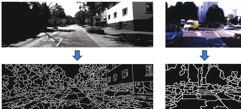
Figure 4.2 – Examples of image segmentation based on the Watershed transform (Vitor et al., 2013), using the KITTI flow benchmark (Geiger et al., 2012) (on the left) and the same stereo vision camera from APACHE (on the right).
