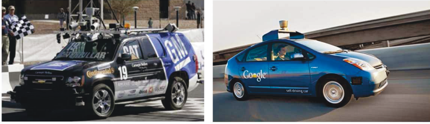
Figure 1.1 – Examples of car-like robots, where on the left is the Boss (Urmson et al., 2008), winner of the DARPA Urban Challenge and on the right is the Google Car (Guizzo, 2011).
