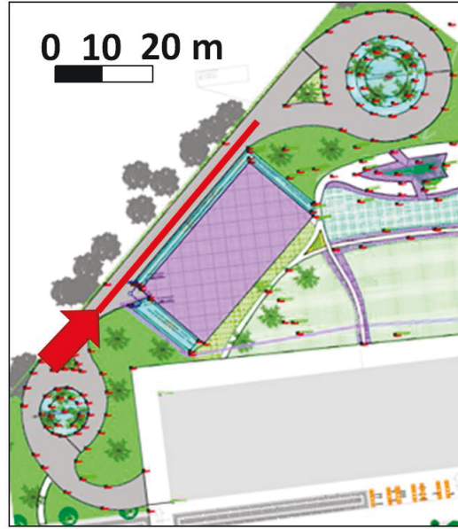
Figure 5.10 – Robot course (red line) for the local navigation experiments at the SEVILLE test track. All experiments start in the arrow.
