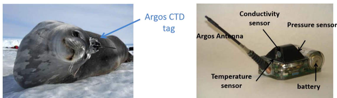
Figure 1.12. Weddell seal equipped with a CTD-SRDL tag (left) (Conductivity Depth Temperature – Satellite Related Data Logger) and details of the sensors on the tag (right)
