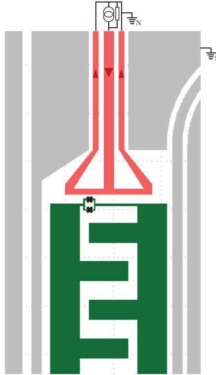
Figure 3.14: Design of our flux lines. The colors are only given for The qubit is in green while the flux line is in red. The ground symbol “S” (“N”) represents connection to the main ground via superconducting (normal) material.
