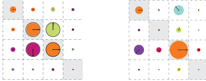
Figure 2.26: Two-qubits tomography after a \sqrt{iSWAP} gate (a) and an iSWAP gate (b) starting from state |ge\rangle . The circle sizes represent absolute values |\rho_{ij}| whereas the arrows the colors both represent the corresponding phases \arg(\rho_{ij}) .
