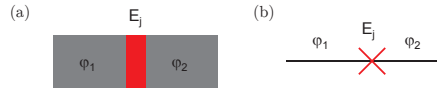
Figure 2.2: Josephson junction. (a) The two superconducting electrodes are in gray while the insulating barrier is show in red. (b) electrically equivalent circuit
