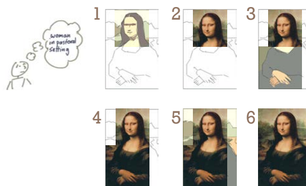
Figure 3.3: Incremental and Iterative Development
