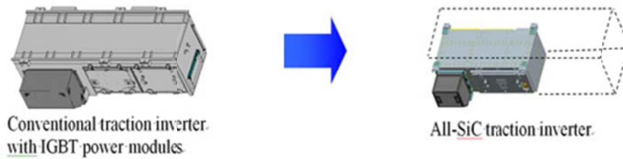
Fig. 2.5 Size reduction of all-SiC inverter compared to conventional inverter [5]
