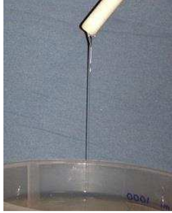
Figure 3.6: Photograph of the fluid filament formed in an aqueous solution of 7 wt.% of PEG and 1000 ppm of PEO. The diameter of the stick is 8 mm.
