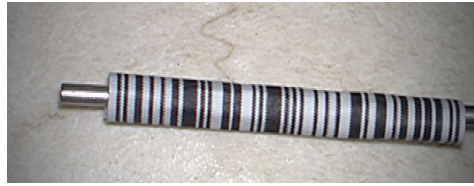
Figure 8.5: Illustration of an EAN barcode placed on a surgical instrument.
