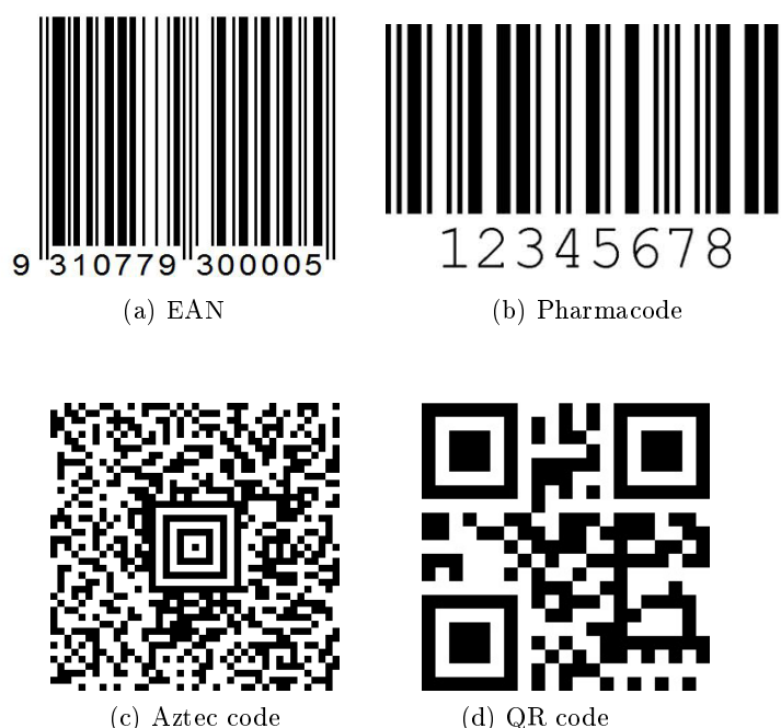
Figure 8.4: Examples of barcode markers. First row: one-dimensional, second row: two-dimensional.
