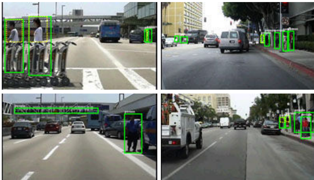
Figure 2.1: Caltech-USA data-set examples. Annotations: green bounding boxes for full pedestrians and dotted yellow bounding boxes for visible pedestrian parts.
