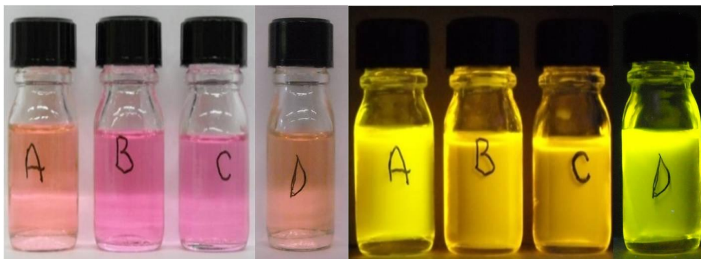
Fig. 51. Visible (left) and UV 365 nm (right) photos of 10^{-3} mol L -1 tetrazine 1 (A), 2 (B), 3 (C) and 4 (D) in ACN
