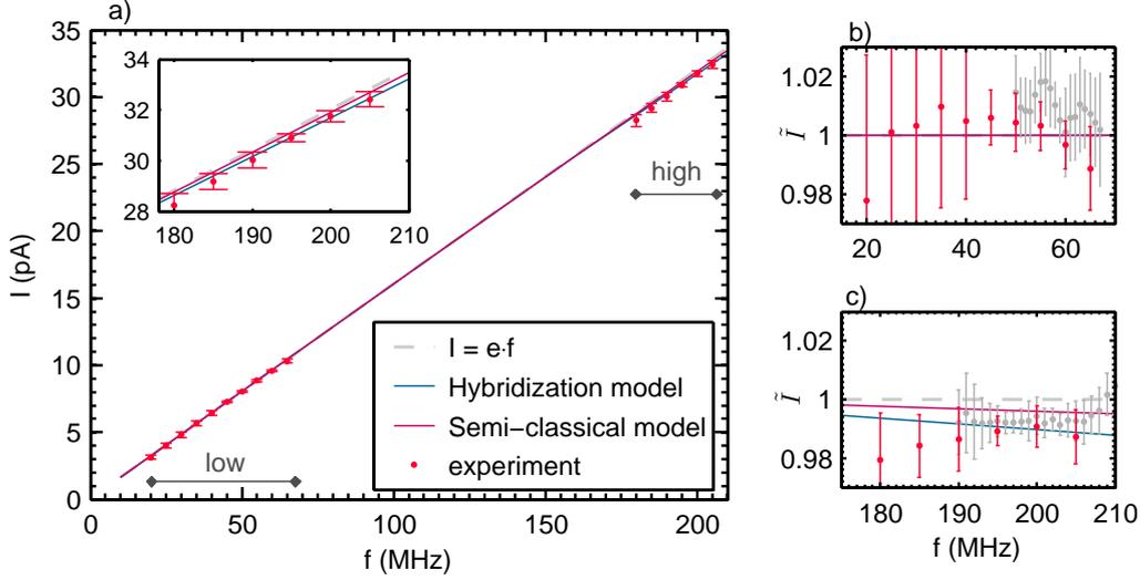
**Figure 6.7:** a) Turnstile current at optimal bias (average over modulation amplitude) as function of the modulation frequency (sine wave, device D). b,c) Current accuracy in the low (b) and high (c) frequency regime, obtained with a sine wave (magenta) and square wave (grey) modulation signal. (solid line give the theoretical prediction based on a semi-classical model (magenta) or 'hybridization' model (blue).)
