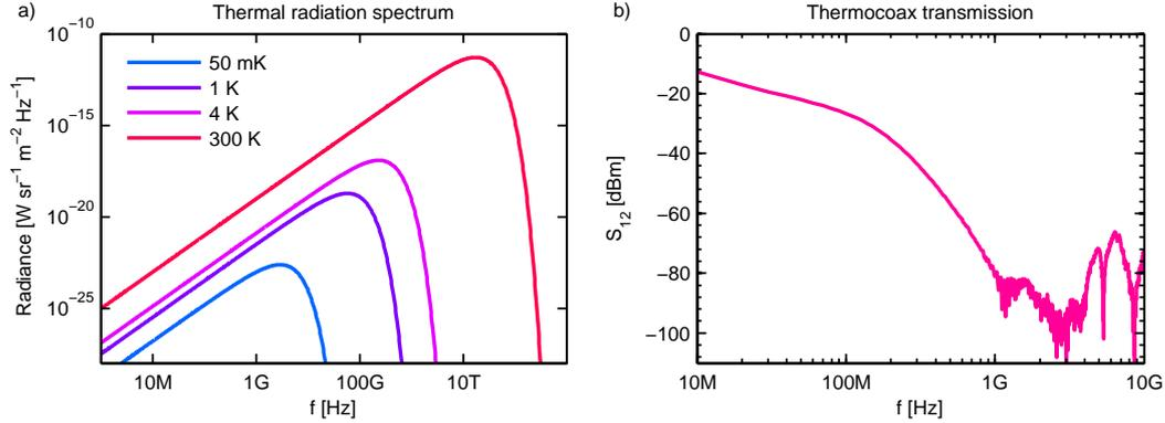
**Figure 2.3:** a) The thermal radiation spectrum at various relevant temperature. At 50 mK the thermal radiation peaks at about 1 GHz. b) Measured transmission of a 2 meter long thermocoax wire. The attenuation becomes maximal above 1 GHz.
