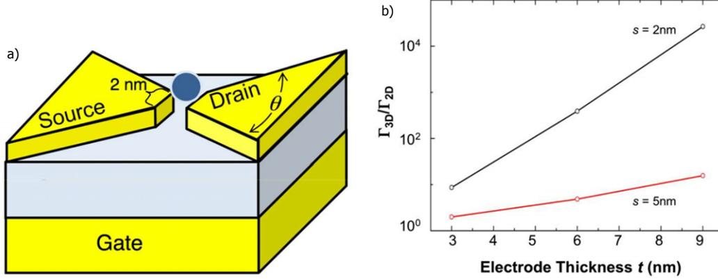
**Figure 1.9:** Finite element simulations show that the gate coupling strongly depends on the geometry of the leads i.e. the sharper the apex angle,  $\theta$  (a) of the contacts, the larger the coupling. (b) The difference in gate coupling (expressed by the ratio) between a 3D system ( $\theta = 120^\circ$ ) and a 2D system ( $\theta = 180^\circ$ ) increases with the thickness of the contacts. (Extracted from [23])
