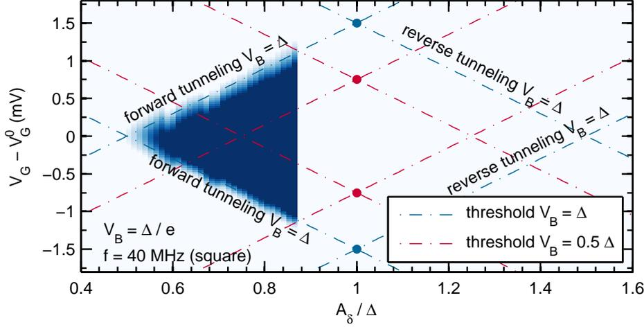
**Figure 6.14:** Turnstile current map as a function of gate detuning and modulation amplitude. The turnstile current appears as a diamond enclosed by four threshold lines of which only a small part is measured.
