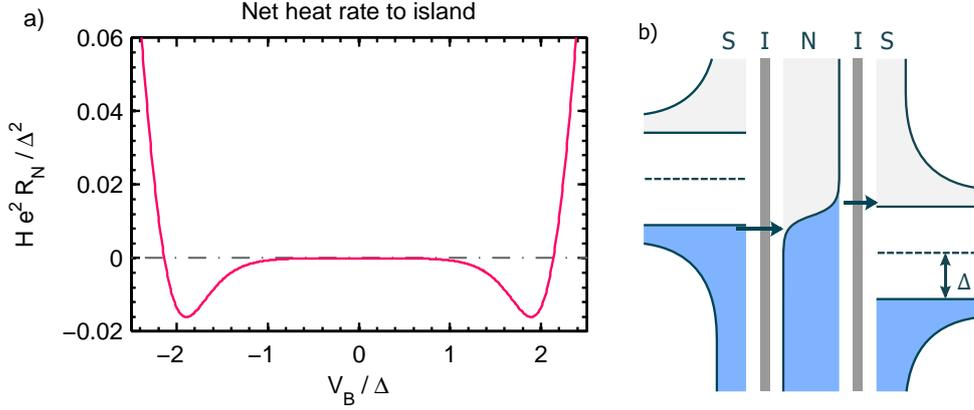
**Figure 3.4:** a) Net heat flow out of the normal island as function of  $V_B$ . Negative flow indicates electronic cooling of the island. ( $T_{base} = 200$  mK,  $E_C = 0.7$  meV,  $R_N = 33$  k $\Omega$ ) b) Heat can be removed from the normal part of an superconductor-normal metal tunnel junction when the applied bias is below  $\Delta$ .
