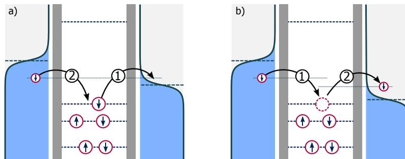
**Figure 3.11:** Higher order tunnel processes are leading when sequential tunneling is blocked by the charging energy. In second order processes, known as cotunneling, electrons can tunnel to and from the quantum dot, even if energy conservation is temporarily violated, provided that a second event 'restores' the quantum dot state. Cotunneling can be both elastic (a) or inelastic (b).
