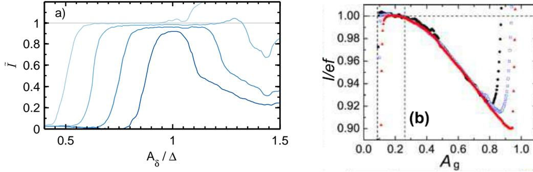
**Figure 6.9:** a) Normalized turnstile current as function the modulation amplitude of a square wave signal measured at several bias positions ( $eV_B/\Delta = 0.25, 0.50, 0.75, 1$ ). The backtunneling onset is clearly visible by the sudden decrease in current. ( $f = 56$  MHz, device C) b) Similar measurements in the SINIS device show a different signature of the backtunneling (Extracted from [71]).
