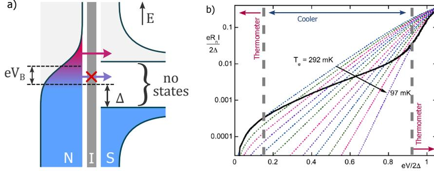
**Figure 3:** a) Energy schematic of a normal metal - insulator - superconductor tunnel junction. b) Experimental current - voltage relation of a low impedance NIS junctions (black line) as a function of the applied bias. Dotted lines give the calculated current - voltage relation of a NIS junctions assuming various fixed electron temperatures in the normal part. (extracted from [123])
