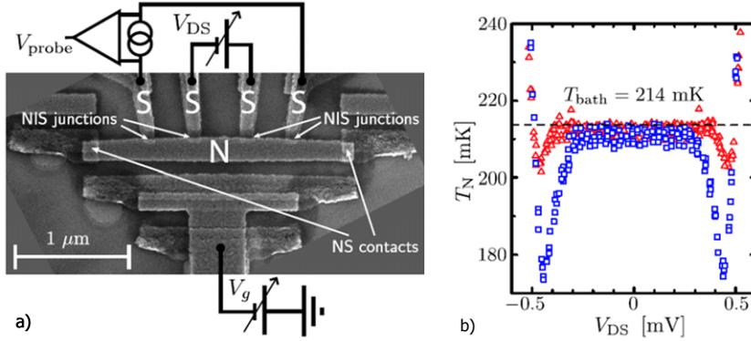
**Figure 4:** a) Scanning electron microscope image of a heat SINIS heat transistor. Additional SIN junctions serve as local thermometers. b) Electron temperature of the normal island as function of the bias when the gate is open (blue) and closed (red). (extracted from [132])
