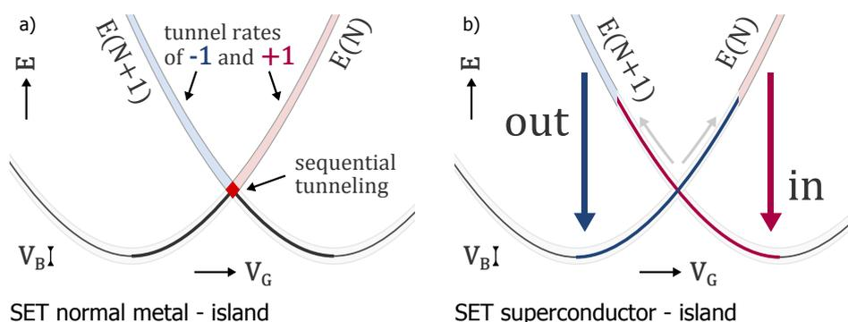
**Figure 5.1:** Single electron transistor charge states as function of the gate. a) Overlapping tunnel rates for adding (red) and removing (blue) electrons from the center island results in sequential tunneling. b) The gap in superconducting leads suppresses the tunnel rates around charge degeneracy and introduces hysteresis in the charge states which is exploited in electron turnstile devices.
