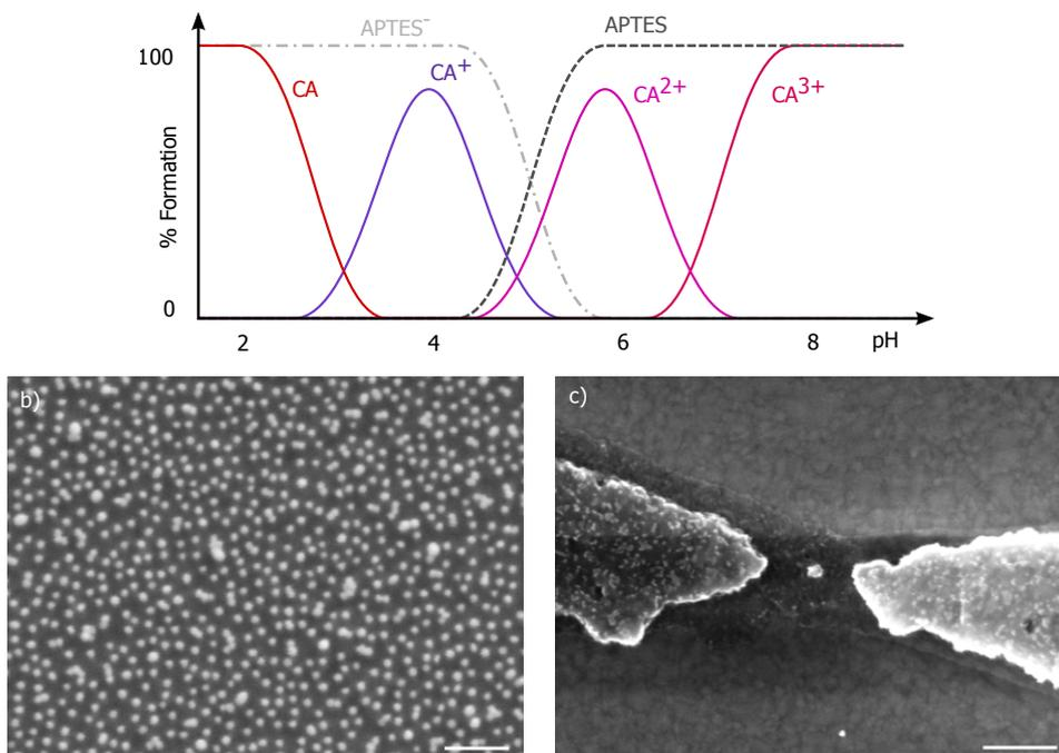
**Figure 1.13:** a) Speciation curves of APTES and citric acid (CA) as a function of the solution pH give the percentage of formation in a solution. b,c) Gold nano-particles deposited using the APTES self-assembly process with two solution acidities. A low solution pH (2-3) results in a dense GNP distribution (b), while a neutral pH (7) leaves APTES uncharged which results in a low density (c). Scale bar represent 100 nm.
