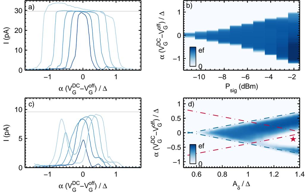
**Figure 6.4:** a) Example traces of the current as function of the center gate position measured with several modulation amplitudes  $P_{sig} = -10, -8, -6, -4, -2$  dBm. b) Turnstile current map constructed from several center gate traces measured with varying modulation amplitude. ( $V_B = 3/2\Delta$ , sine wave, device D) c, d) Similar measurements at  $V_B = \Delta$ . (square wave, device D)
