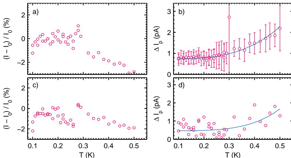
**Figure 6.11:** Turnstile current accuracy at  $V_B^{opt}$  (a, c) and current drop over the plateau (c, d) as function of the cryostat base temperature. The data presented in (a,b) are the average values of all measured modulation amplitudes, while (c,d) only show the data at optimal modulation amplitude. The solid lines are a guide to the eye. (device C,  $f = 56\text{MHz}$ , square wave)
