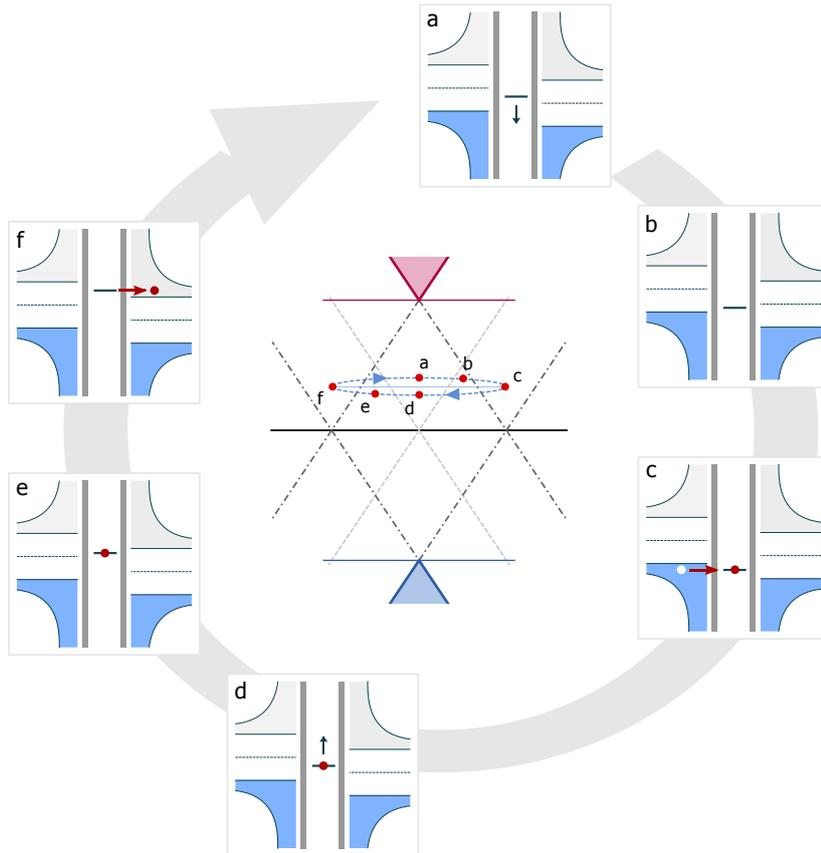
**Figure 5.2:** A system in which a single level is coupled to two superconducting leads can be used as a single electron turnstile. Driving the level in a cyclic manner through the charge degeneracy region at constant bias generates a quantized current which is equal to  $ef$ . The level trajectory corresponds to a horizontal movement in the conductance map of a quantum dot. During each cycle the level passed through various states illustrated by the chemical potential diagrams (a-f).
