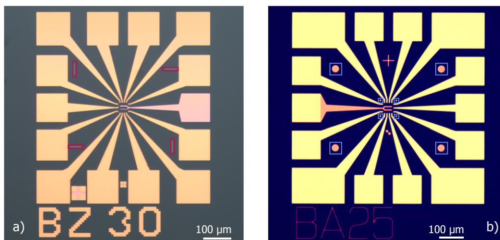
**Figure 1.6:** The two optical (i.e. DUV (a) and laser (b)) lithography designs, are very similar. In the design for laser lithography we have implemented 8 circular markers (highlighted in pink) that are used for the calibration of writefields and the automatic realignment during e-beam lithography. The circular markers replace the line markers (highlighted in blue) in the DUV design.
