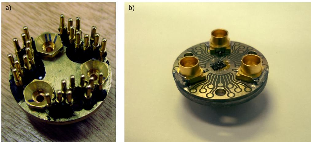
**Figure 2.6:** The sample stage (a) is made of a thick brass disk on which 27 spring-pin connectors and 3 SMP receptacles are mounted. The three SMP connectors ensure a good alignment of the 27 spring-pins with respect to the sample carrier (b).
