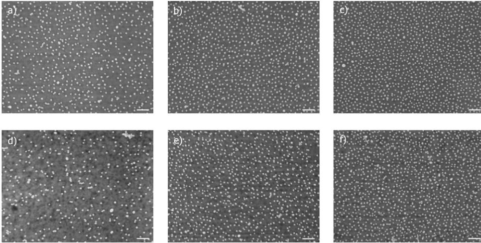
**Figure 1.15:** Scanning electron microscope images of gold nanoparticles (12 nm) deposited with (a, b, c) and without (d, e, f) the use of a self assembling monolayer and during a varying time in a gold nano-particle suspension. Overall the particle dispersion of the samples with a self assembling monolayer have high particle density and are more homogeneous. However the difference in particle density becomes less when the time spend in the gold nano-particles suspension increases.
