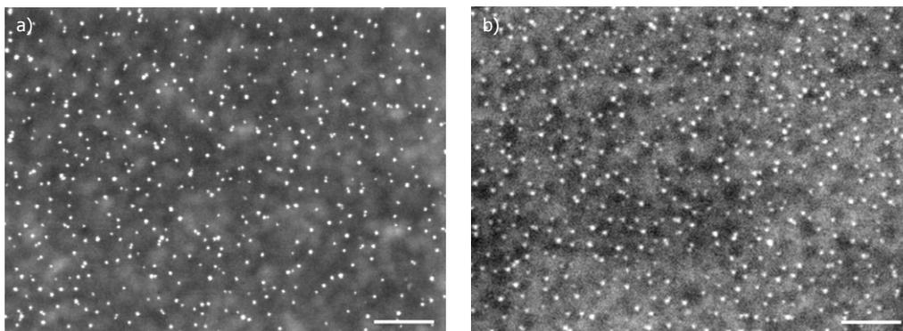
**Figure 1.11:** Scanning electron microscope images of gold nanoparticles (5 nm) distributed on a substrate after spincoating (a) and drop-casting (b). Under equal conditions the drop-casting technique gives better results than spincoating. The scale-bar in both images represent 50 nm.
