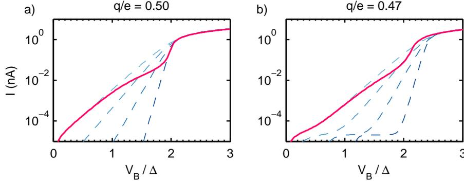
**Figure 3.5:** Electronic cooling of the normal island in a superconducting SET is visible in the sub-threshold current. The solid lines is the numerical self consistent solution of the master equation and heat balance equation. The dashed lines give the  $I(V_B)$  curves of the system at constant normal island temperature (isotherms). (radius = 100 nm,  $\kappa = 2.3 \cdot 10^9$ ,  $R_N = 33\text{k}\Omega$ ,  $T_{bath} = 200$  mK,  $E_C = 0.7$  meV)
