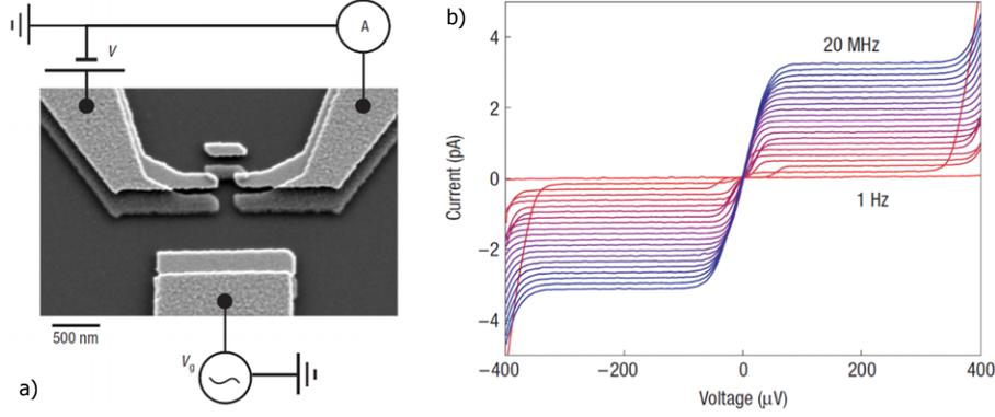
**Figure 5.5:** a) Scanning electron microscope (SEM) image of a hybrid SET single electron turnstile with a relatively large island (zero level spacing). b) Quantized current at varying modulation frequencies as function of the device bias measured by Pekola *et al.* [117].
