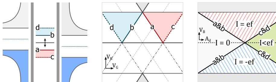
**Figure 5.3:** A single level electron turnstile can operate in three regimes of signal amplitude which depend on the source-drain bias. At small signal amplitude the level remains between the position  $a$  and  $b$  such that  $I = 0$ . The turnstile current will be optimal when  $\Delta - V_B/2 < A_g < \Delta + V_B/2$ . When the amplitude becomes larger, the turnstile current will deteriorate due to backtunneling events.
