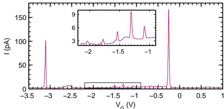
**Figure 4.2:** Example DC current trace ( $V_B = 3$  mV,  $T = 4$  K) as a function of the gate voltage. The  $I(V_G)$  curve shows sharp Coulomb oscillations. Often there are peaks of various shapes and heights present, which might indicate the co-existence of multiple gold-nanoparticles inside the nano-gap.
