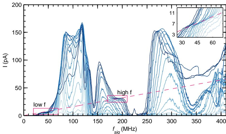
**Figure 6.1:** DC turnstile current (device D) as function the sine wave modulation frequency measured at varying modulation amplitude (increasing from bright to dark). The dashed magenta line gives the theoretical turnstile current  $I = ef$ . ( $T = 90$  mK,  $eV_B = 3/2\Delta$ ,  $A_{sig} = -18$  to  $-2$  dBm)
