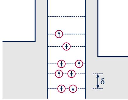
**Figure 3.7:** The small size of a quantum dot confines the electrons in a small space. This results in a non-zero level spacing. Each level can be filled by zero, one (spin up or down) or two (spin up and down) electrons.
