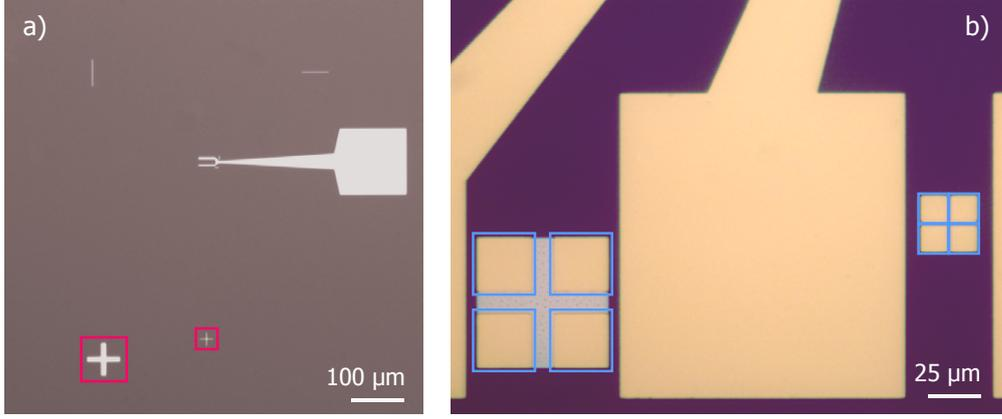
**Figure 1.3:** The alignment of different lithography steps is achieved by adding complementary markers to the design of subsequent layers. The gate layer (a) contains little crosses (highlighted in pink) that next to be aligned with the four little squares (highlighted in blue in (b)) in the next layer.
