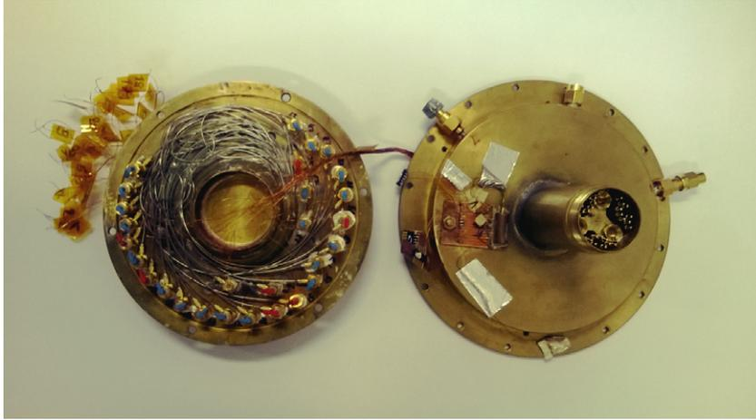
**Figure 2.5:** The cold stage consists of two chambers separated from each other by a solid brass disk through which the 27 thermocoax wires go (left). The upper part of the cold stage (right) contains the sample stage.
