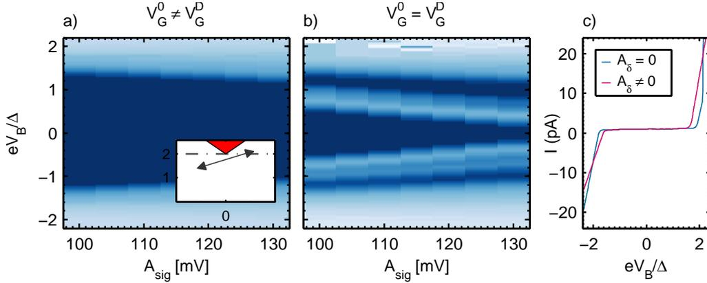
**Figure 6.8:** Differential conductance maps as function of bias and modulation amplitude measured with a large (a) and zero (b) detuning from the gate offset position (square wave,  $f = 60$  MHz, device C). c) Example current traces as a function of bias at charge degeneracy illustrating the cross-talk between the AC gate modulation signal and bias voltage.
