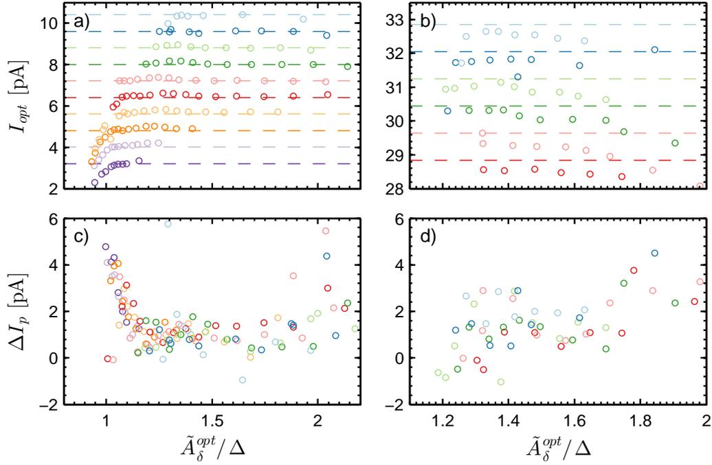
**Figure 6.6:** Turnstile current along the line of minimal differential conductance at the current plateau (a, b) and the current drop  $\Delta I_p$  (c, d), as function of  $A_\delta$  for a set of frequencies (5 MHz steps) in the low (a: 20 - 65 MHz) and high (b: 180 - 205 MHz) modulation regime (sine wave, device D).
