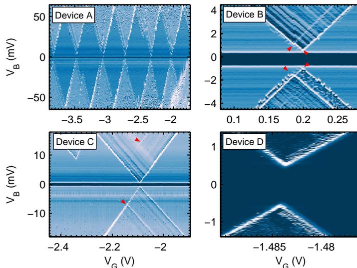
**Figure 4.3:** Color maps of the differential conductance measurement in four devices (A, B, C, D) at base temperature ( $T \approx 80$  mK). Coulomb diamonds measured in most devices (denoted by an asterix in table 4.1), e.g. (b-d), extend beyond the scope of the measurements. Additional slanted lines (indicated by red arrows) outside the Coulomb diamonds observed in some devices indicate single quantum dot levels (excitations) with an energy spacing that varies between 2 and 10 meV.
