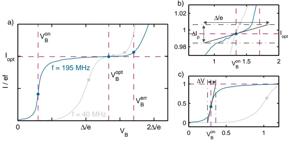
**Figure 6.5:** The turnstile operation as function of bias (sine wave,  $f = 195$  MHz and 40 MHz) is characterized in terms of current onset, optimal bias and error bias. The current plateau is characterized by the current variation  $\Delta I_p$  and the onset width  $\Delta V$ .
