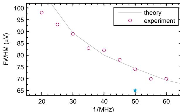
**Figure 6.16:** Full-width-half-maximum (FWHM) values of the differential conductance peaks presented in figure 6.15 for sine (circles) and square (star) wave modulation signal. The solid grey curve represents the theoretical estimation based on the adiabatic model.
