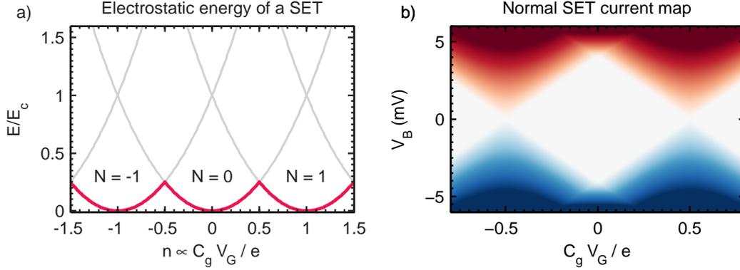
**Figure 3.2:** a) The electrostatic energy of the island depends on the number of additional charges on the island. For each value of the additional charge, the electrostatic energy is a parabolic function of the gate induced charge. The red curve denotes the island ground state. b) The current map, i.e.  $I(V_B, V_G)$ , of a single electron transistor shows diamond shaped areas in which the current is zero. ( $T = 100$  mK,  $E_C = 2.0$  meV)
