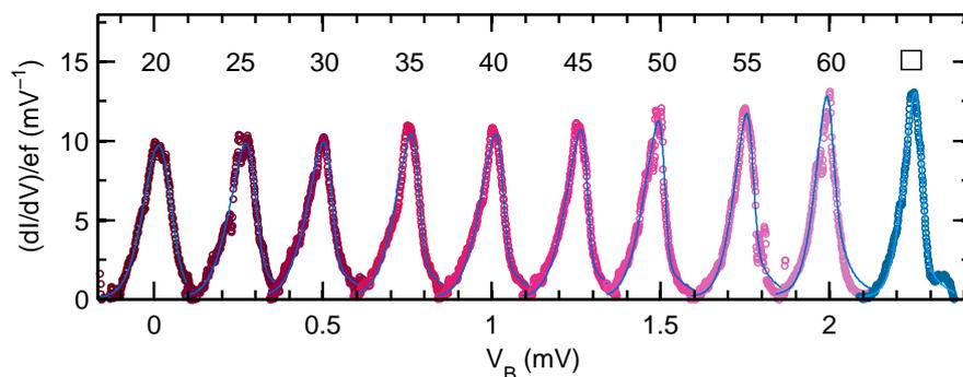
**Figure 6.15:** Normalized differential conductance peaks of the plateau onset measured at several modulation frequencies (20-60 MHz) of a sine wave (shifted by 0.25 mV). The modulation amplitude of each onset is adapted such that the onset takes place at  $V_B \approx \Delta$ . The rightmost curve shows the differential conductance of the onset measured with a square wave modulation signal ( $f = 50\text{MHz}$ ). (device D)
