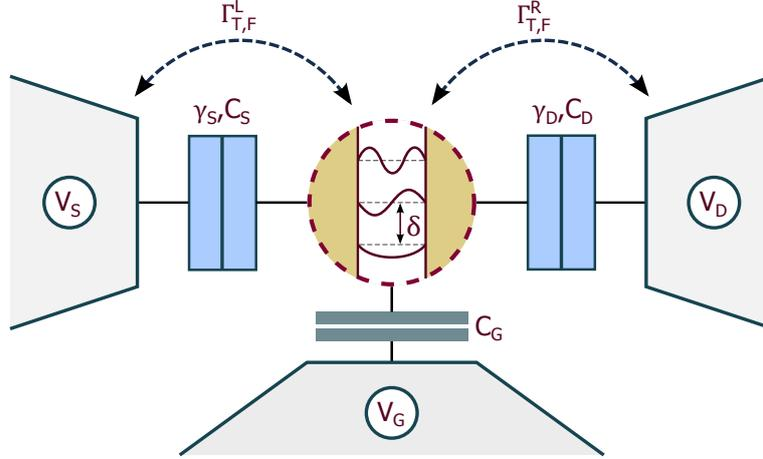
**Figure 3.1:** In a single electron transistor, a small metallic island ( $\delta = 0$ ) or quantum dot ( $\delta \neq 0$ ) is connected by three terminals. Current can pass through the device by two tunnel junctions that are characterized by their capacitance  $C_{S,D}$  and transparency  $\gamma_{S,D}$ . The third electrode (gate) is only capacitively coupled to the center and allows independent manipulation of the electrostatic potential of the island.
