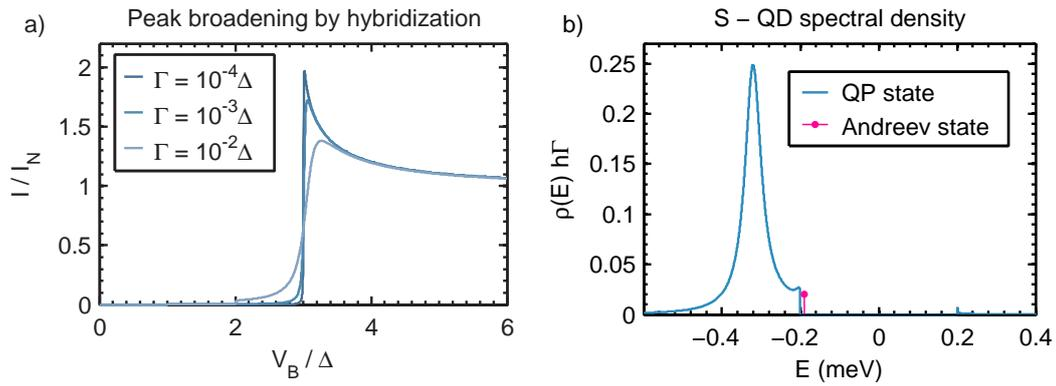
**Figure 3.12:** a) Current through a single level coupled to two superconductors as a function of the applied source-drain bias calculated with eq. (3.23). Increasing tunnel coupling softens the coherence peak. b) The spectral density of a single level is significantly altered when it is coupled to a superconducting density of states, i.e. (1) there is a broadened quasi-particle (QP) state and (2) a persistent discrete state (Andreev state) that remains bound in the superconducting gap.
