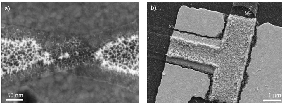
**Figure 1.16:** The aqueous gold nano-particle solution has a detrimental effect on the aluminium electromigration junctions. (a) The scanning electron microscope image of the electromigration junction shows that the ionic environment attacks and partly dissolve the aluminium. (b) At the connection between the aluminium junctions and the gold contact leads the two metals interact, possibly forming an intermetallic compound. This process is possible enhanced by the ionic environment.
