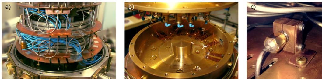
**Figure 2.2:** a) 27 measurement wires are divided into three capillaries, each filled with Eccosorb [31]. Capillaries shield the wires from radiation, while the Eccosorb filters the high frequency noise on the lines. b) Between the capillaries and the Thermocoax[140], the wires are thermalized at base temperature inside a massive shielded box. c) To thermalize the center conductor of the RF lines, we use -10 dBm attenuator at 4K, solidly clamped in copper.
