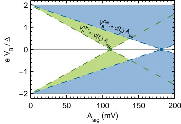
**Figure 6.3:** Theoretical turnstile current diagram as a function of signal amplitude and bias for two different operation frequencies. Dashed lines corresponding to the current onset, construct regions of quantized current (hatched areas). The slopes of the current onset is affected by the frequency dependent signal transmission  $c(f)$ .
