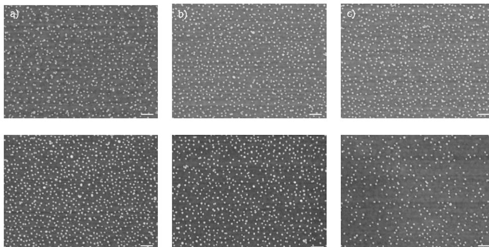
**Figure 1.14:** Scanning electron microscope images of gold nanoparticles (12 nm) deposited using a self assembling monolayer created with varying silanization parameters. The oxygen plasma time (a, b, c) (APTES dose = 4 sccm) plasma time has little significant effect on the particle density. However with increasing APTES dose (d, e, f) (plasma time = 30 s) their appears to be a little decrease in particle density. The scale bars represent 100 nm.
