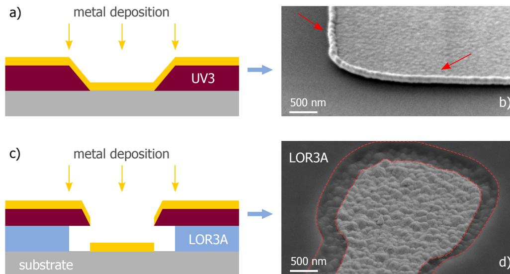
**Figure 1.2:** The bilayer resist technique (c, d) can be used to prevent the formation of upstanding edges (denoted by the arrows in b) after lift off, which can occur when using a single resist layer (a, b). The undercut in the bilayer resist ensures that the metallic film on the substrate will never extend over the lower resist layer. The red dotted line in (d) shows the separation between the lower resist layer (LOR3A) and the structure.
