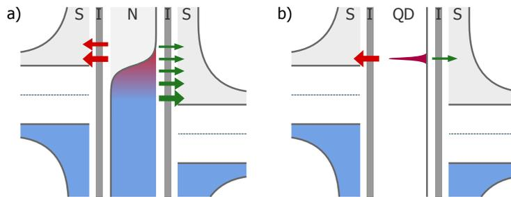
**Figure 6.10:** Energies schematic illustrating the energy windows available for forward tunneling (green) and backtunneling (red) in a single *electron* turnstile (a) and a single *level* turnstile (b).
