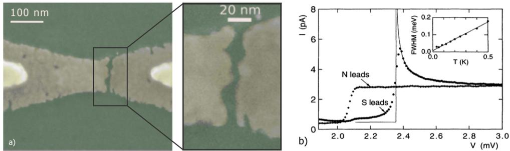
**Figure 5:** a) Scanning electron microscope image of a nano-gap created by the electromigration process. (extracted from [128]. b) Current-voltage relation of a quantum dot contacted by superconducting electrodes in normal and superconducting state. (extracted from [124])
