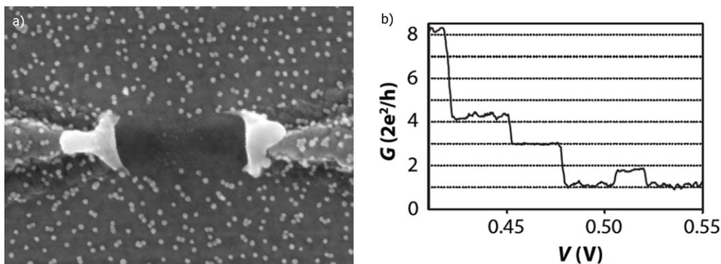
**Figure 1.17:** (a) A scanning electron microscope image of a fused electromigration junction. When during electromigration the local temperature becomes too high the process spins out of control and the junction 'explodes'. (b) When the electromigration process develops controlled and without excessive heating the junction conductance steadily decreases until it becomes quantized just before it enters the tunnel-regime. (extracted from [127])
