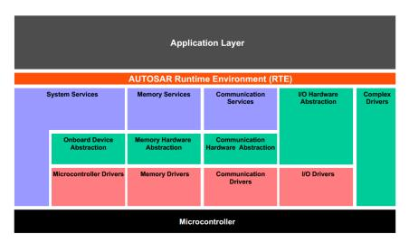
FIGURE 5.4 DESCRIPTION OF AUTOSAR LAYERS AND STACKS OF THE BASIC SOFTWARE (AUTOSAR, 2015)
