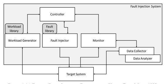
FIGURE 1.4 A TYPICAL FAULT INJECTION ENVIRONMENT (HSUEH, TSAI, & IYER, 1997)
