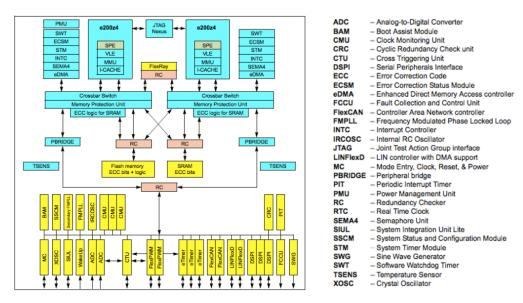
FIGURE 5.3 SPC56EL70 ARCHITECTURE (STMICROELECTRONIC, 2013)
