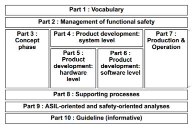
FIGURE 1.1 THE TEN PARTS OF THE ISO 26262 (ISO 26262, 2011)
