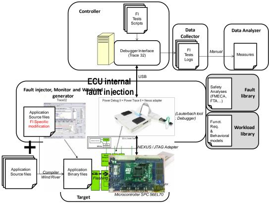
FIGURE 6.1 FAULT INJECTION ENVIRONMENT
