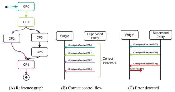
FIGURE 5.7 AUTOSAR WDGM: CONTROL FLOW MONITORING EXAMPLE
