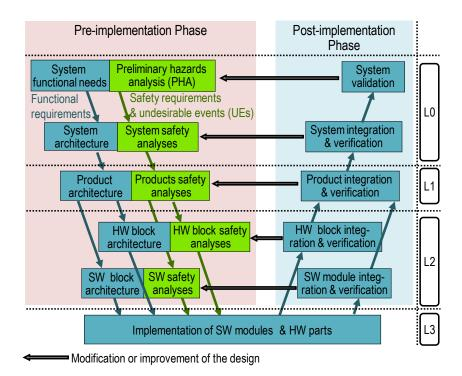
FIGURE 2.2 V-CYCLE DEVELOPMENT PROCESS AND TERMINOLOGY USED
