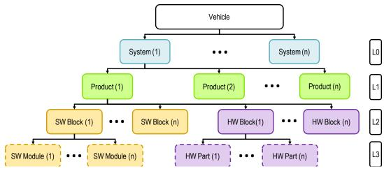
FIGURE 2.1 ARCHITECTURAL ABSTRACTION LEVELS OF A VEHICLE
