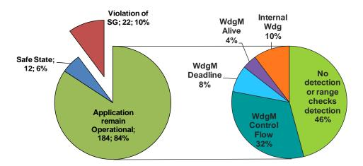
FIGURE 6.5 GLOBAL RESULT OF THE VIOLATION OF THE SAFETY REQUIREMENTS AND THE TRIGGERED SAFETY MECHANISMS (218 EXPERIMENTS)
