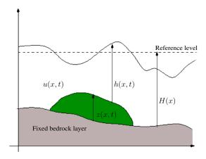
Figure 2: The one-dimensional sketch of shallow water with a sediment layer.
