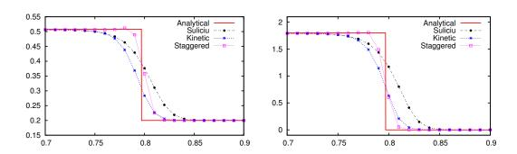
Figure 1.5: Dam break on a wet bed. Water height (left) and velocity (right) around the shock at time t = 0.1. The number of cells is 100.
