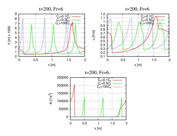
Figure 5.16: The comparison of h, u and  $\Phi$  in various  $C_f$  at final time t=200.
