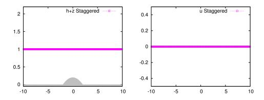
Figure 1.11: The steady state at rest over a bump. Water level (left) and velocity (right) at final time. The number of cells is 300.
