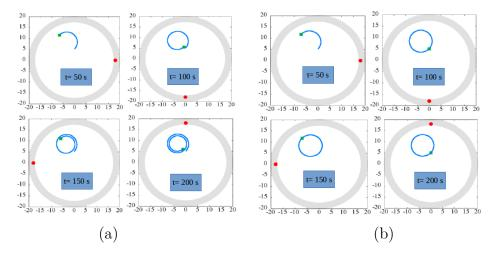
Figure 2.2: The parcel trajectory in a rotating frame. (a) Trajectory from the implicit Euler scheme. (b) Trajectory from Crank-Nicolson scheme. The red point denotes the reference location in the fixed frame of reference.
