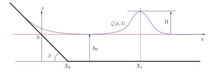
Figure 5.17: The sketch of runup of solitary wave.
