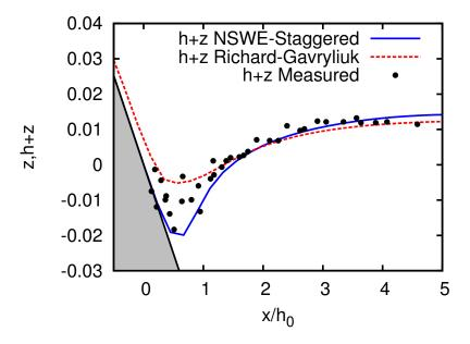
Figure 5.24: The comparison of surface profile between standard shallow water equtaions using staggered grid scheme and Richard-Gavrilyuk model using collocated HLLC flux at various final time step  $t = 70t_0$  in the zoom part.
