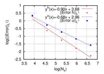
Figure 3.2: The convergence rate of discrete  $L^1$ -norm error of h and u in various grid points  $N_x$ . The functions  $y^h(x)$  and  $y^u(x)$  are obtained from data fitting of  $L^1$ -norm error of h and u respectively using the nonlinear least-squares method.
