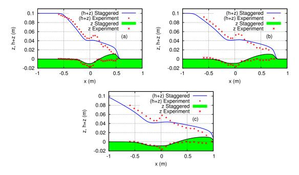
Figure 4.8: Dam-break over a granular bed. Comparison between numerical computations and experimental data of the water level and sediment at subsequent times (a)  $t = 5t_0$ , (b)  $t = 7.5t_0$  and (d)  $t = 10t_0$  with  $t_0 = \sqrt{gh_0} \approx 0.101$ . Meyer-Peter & Müller's formula (4.5) is used in this computation.
