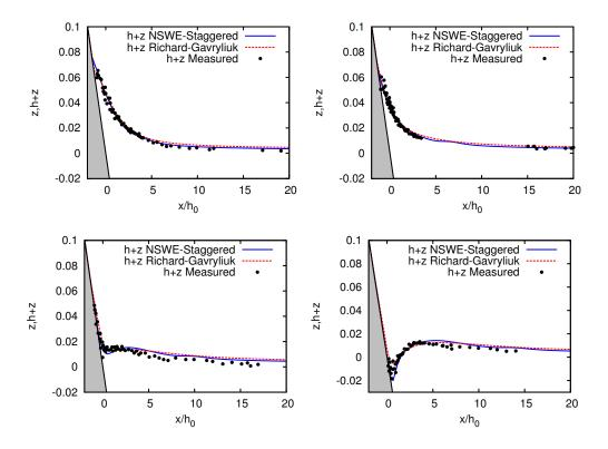
Figure 5.23: The comparison of surface profile between standard shallow water equtaions using staggered grid scheme and Richard-Gavrilyuk model using collocated HLLC flux at various final time steps. The time steps are provided from  $t = 55t_0$  to  $t = 70t_0$  with 5 increments and the initial wave  $H/h_0 = 1.85 \times 10^{-2}$ . The coefficients  $C_r$  and  $C_f$  in Richard-Gavrilyuk model are set to be 0.01 and 0.006 respectively.
