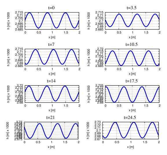
Figure 5.14: The evolution of roll-waves by Richard-Gavrilyuk model using HLLC solver with several times. The parameters values are  $\epsilon=0.5\%,\,k=5\pi,\,C_f=0.048/8,\,q_0=0.001m^2s^{-1},\,\phi_0=0.02,\,C_r=0.5C_f$  and  $F_r=2$ .
