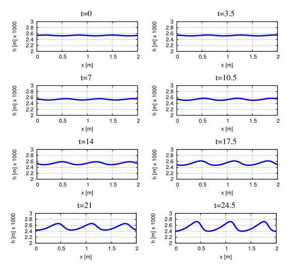
Figure 5.15: The evolution of roll-waves by Richard-Gavrilyuk model using HLLC solver with several times. The parameters values are  $\epsilon=0.5\%,\,k=5\pi,\,C_f=0.048/8,\,q_0=0.001m^2s^{-1},\,\phi_0=0.02,\,C_r=0.5C_f$  and  $F_r=2.5.$
