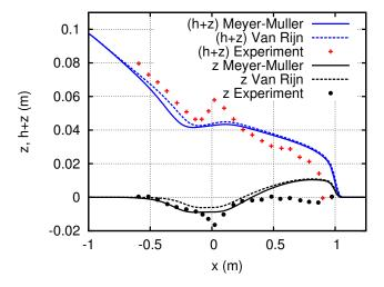
Figure 4.7: Dam-break over a granular bed. Comparison between numerical computations and experimental data. The calculated water level and sediment profiles at final time  $t = 10t_0$ ,  $t_0 = \sqrt{gh_0} \approx 0.101$  with bedload following Meyer-peter & Müller's (4.5) and Van Rijn's (4.9) formulas.
