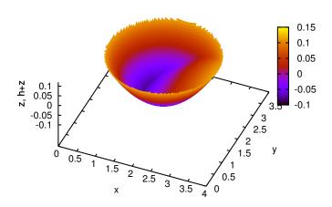
Figure 1.13: Oscillations in a paraboloid. Water level h+z at time  $t=3\frac{2\pi}{\omega}$ . The number of cells is  $100\times 100$ .
