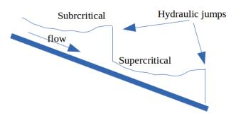
Figure 5.7: Sketch of roll waves down an inclined open channel
