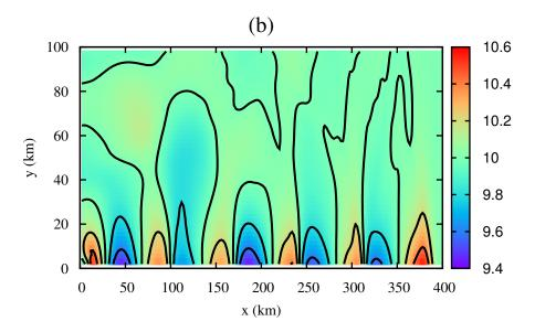
Figure 2.8: Surface wave contours at final time t=10.6 hours. (a) Without Coriolis force and (b) with Coriolis force.
