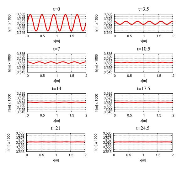
Figure 5.10: The evolution of roll-waves by staggered scheme with several times. The parameters values are  $\epsilon=0.5\%,\ k=5\pi,\ C_f=0.048/8,\ q_0=0.001m^2s^{-1},$  and  $F_r=1.5.$
