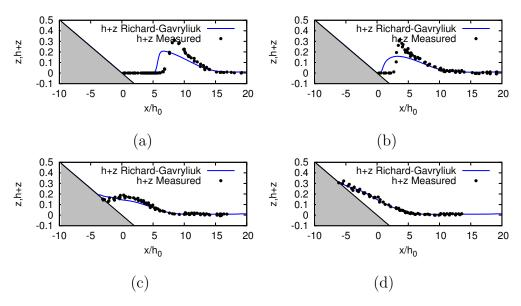
Figure 5.20: The surface profile of Richard-Gavrilyuk model at  $t = 15t_0$  (a),  $t = 20t_0$  (b),  $t = 25t_0$  (c), and  $t = 30t_0$  (d). The coefficients  $C_r$  and  $C_f$  are set to be 0.01 and 0.006 respectively.
