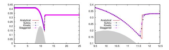
Figure 1.7: Transcritical flow with shock. Water level h + z at time t = 200. The right figure is a zoom of the left figure. The number of cells is 200.
