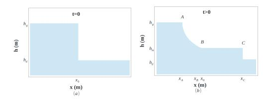
Figure A.1: Dam break on wet bottom
