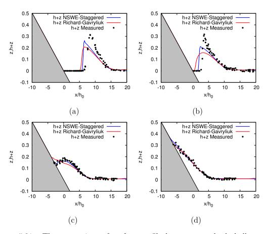
Figure 5.21: The comparison of surface profile between standard shallow water equtaions using staggered grid scheme and Richard-Gavrilyuk model using collocated HLLC flux at various final times  $t = 15t_0$  (a),  $t = 20t_0$  (b),  $t = 25t_0$  (c), and  $t = 30t_0$  (d). The coefficients  $C_r$  and  $C_f$  in Richard-Gavrilyuk model are set to be 0.01 and 0.006 respectively.
