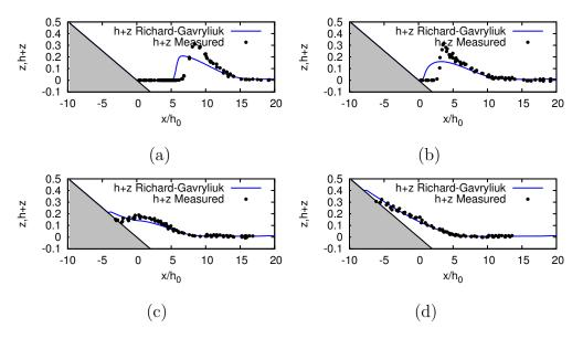
Figure 5.19: The surface profile of Richard-Gavrilyuk model at  $t = 15t_0$  (a),  $t = 20t_0$  (b),  $t = 25t_0$  (c), and  $t = 30t_0$  (d). The coefficients  $C_r$  and  $C_f$  are set to be zero for both.
