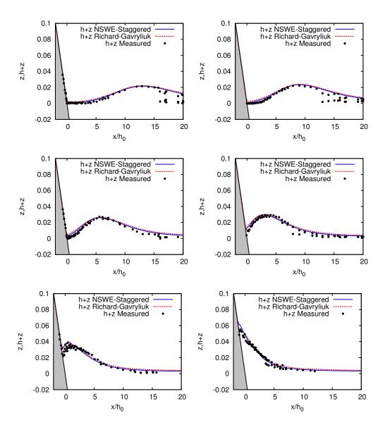
Figure 5.22: The comparison of surface profile between standard shallow water equtaions using staggered grid scheme and Richard-Gavrilyuk model using collocated HLLC flux at various final time steps. The time steps are provided from  $t = 25t_0$  to  $t = 50t_0$  with 5 increments and the initial wave  $H/h_0 = 1.85 \times 10^{-2}$ . The coefficients  $C_r$  and  $C_f$  in Richard-Gavrilyuk model are set to be 0.01 and 0.006 respectively.
