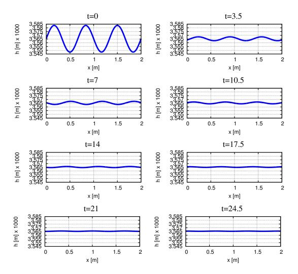
Figure 5.13: The evolution of roll-waves by Richard-Gavrilyuk model using HLLC solver with several times. The parameters values are  $\epsilon=0.5\%,\,k=5\pi,\,C_f=0.048/8,\,q_0=0.001m^2s^{-1},\,\phi_0=0.02,\,C_r=0.5C_f$  and  $F_r=1.5$ .
