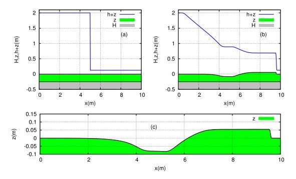
Figure 4.6: One-dimensional erodible dam break. (a) Initial position of dam break problem. (b) Water level h+z and sediment z profiles at final time t=1. (c) Zoom area of sediment profile at final time t=1. In this simulation we used the Grass formula with  $A_g=5\times 10^{-3}$  and m=3.
