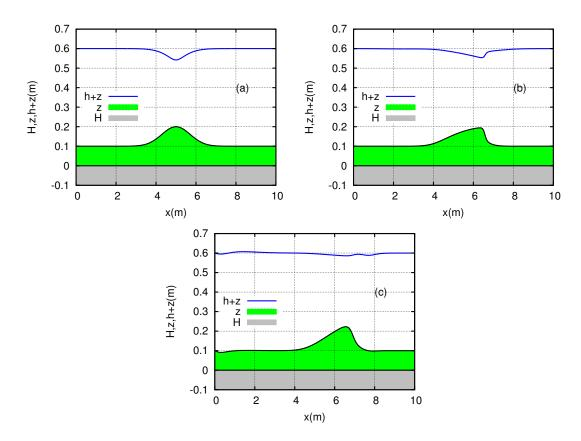
Figure 4.9: Subcritical steady state over a moveable bump. Simulations with sediment discharge of Grass formula with m=3, calculated using 400 mesh points. The profiles of free surface h+z and sediment z (a) at initial time, (b) at time t=10, with parameter  $A_g=5\times 10^{-3}$ , (c) at time t=2.6 with parameter  $A_g=7\times 10^{-2}$ .
