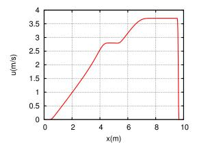
Figure 4.5: One-dimensional erodible dam break. Velocity profile at final time t = 1. In this simulation we used the Grass formula with  $A_g = 5 \times 10^{-3}$  and m = 3.
