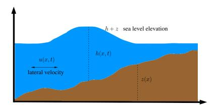
Figure 1: One-dimensional shallow water model.
