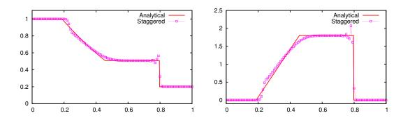
Figure 1.6: Dam break on a wet bed. Water height (left) and velocity (right) at time t = 0.1. The number of cells is 100.
