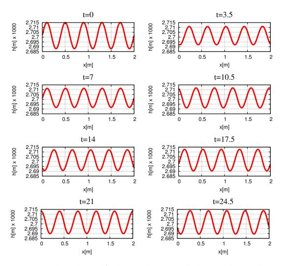
Figure 5.11: The evolution of roll-waves by staggered scheme with several times. The parameters values are  $\epsilon=0.5\%,\ k=5\pi,\ C_f=0.048/8,\ q_0=0.001m^2s^{-1},$  and  $F_r=2.$
