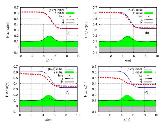
Figure 4.11: Transcritical flow over a granular bump. Water level and sediment profiles with  $A_g = 5 \times 10^{-4}$  at times (a) t=1, (b) t=5, (c) t=15 and (d) t=30.
