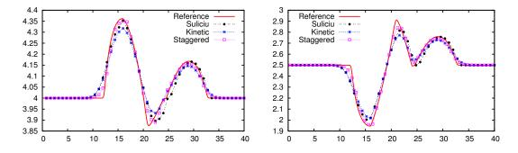
Figure 1.3: Accuracy test. Water level (left) and velocity (right) at final time. The number of cells is 50.
