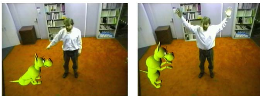
Figure 2.2 – A dog agent able to react to the user's gestures using rules to select between the branches of a decision tree [Blumberg, 1996].
