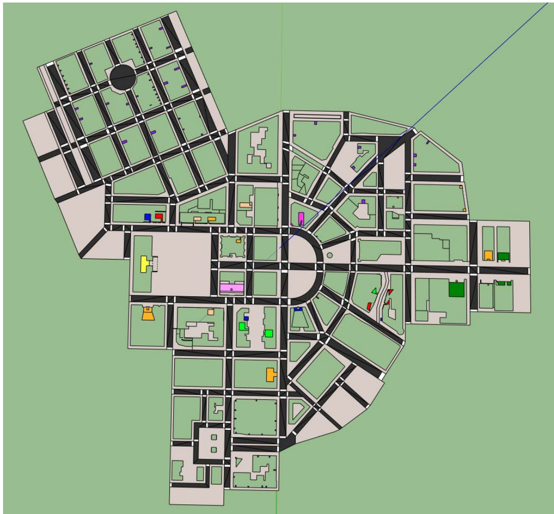
Figure A.1 – Example of an informed geometry of the environment. Navigation surfaces are labelled through the use of textures. For clarity purpose, only the navigation surfaces are shown here.
