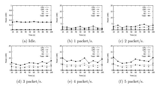
Figure 4.7: Energy consumption in router mode
