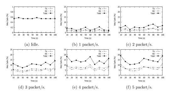
Figure 4.9: Duty cycle in *router mode*
