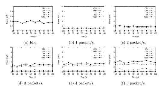
Figure 4.6: Energy consumption in host mode.
