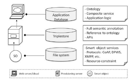
Figure 3.2: Data model in the hierarchical scheme.
