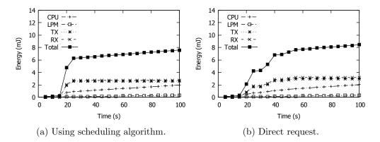
Figure 5.10: Comparison of energy consumption when multiple simultaneous requests are sent to one smart object.
