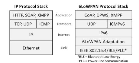
Figure 4.1: IP and 6LoWPAN protocol stack in reference to layers of the TCP/IP networking model.
