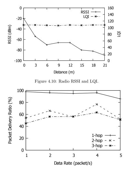
Figure 4.11: Packet Delivery Ratio.
