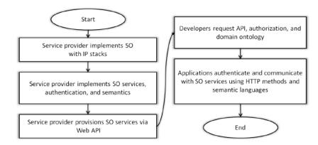
Figure 3.5: Provisioning workflow.
