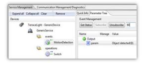
Figure A.3: DPWS Explorer discovers a DPWSim device *TerraceLight* containing an event *MotionDetection* and an operation *Switch*. The green icon next to the *MotionDetection* event indicates that DPWS Explorer is subscribing to the event; once the event occurs, DPWS Explorer will receive the notification, e.g., *Object detected*.
