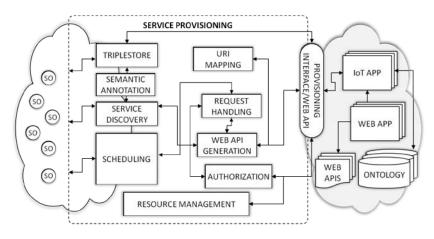
Figure 5.2: Semantic service provisioning architecture.
