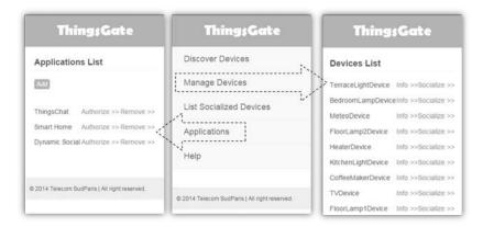
Figure 5.4: Resource Management Web UI in ThingsGate. Manage Device function/menu shows a list of discovered devices in the 6LoWPAN of home network. User can query detailed information or add social data to each device by Info or Socialize hyperlinks associated to each smart object. Applications function/menu help users to authorize IoT applications on Web to use resources in the 6LoWPAN.
