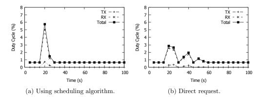
Figure 5.9: Comparison of radio duty cycle when multiple simultaneous requests are sent to one smart object.
