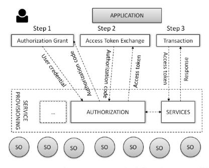
Figure 5.3: 3-step authorization process for IoT applications on Web.
