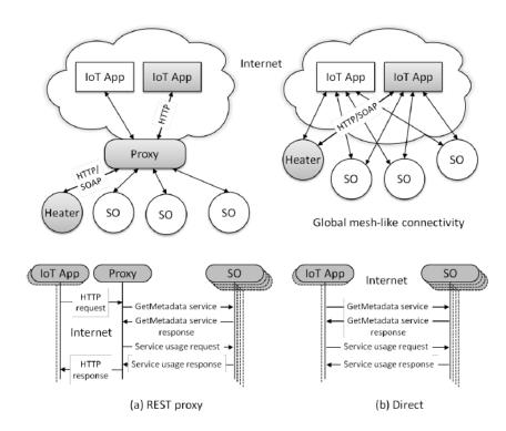
Figure 5.5: Network topology in two cases: (a) Our proposed design configures a proxybased topology with local HTTP/SOAP binding, (b) The original smart objects Profile for Web Services (DPWS) communication configures global mesh-like connectivity for HTTP/SOAP binding. Consequently, the original DPWS introduces higher latency and overhead.
