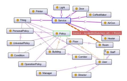
Figure 6.8: Building Ontology graph. The highlighted blocks in the graph show the hierarchy among class *Service* and its subclasses. The dotted line with a label presents a property called *locatedIn* which takes class *Room* as object meaning a service is located in a room.
