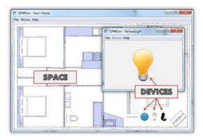
Figure A.1: A home space contains three devices: a generic DPWSim device (blue button), a light bulb, and a coffee maker. A stand-alone device (space with only one device) is a light bulb.
