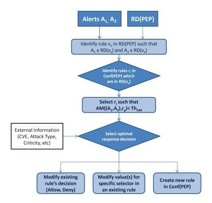
FIGURE 6.2 - Enforcement-based alert correlation workflow with two alerts
