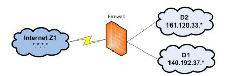
FIGURE 4.5 - Running Example: a network with two zones.
