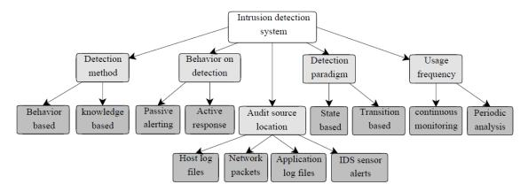
FIGURE 2.3 - Intrusion Detection taxonomy, source [24]. The categorization depends on the detection method, behavior on detection, detection paradigm, usage frequency.
