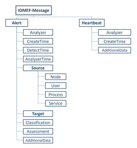
FIGURE 2.4 - IDMEF Alert model. It is composed of two major classes that are the alert class and the heartbeat class. The alert class includes information about the detected attack. The heartbeat class indicates information about the current analyzer's status to managers
