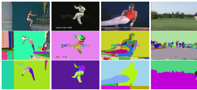
Figure 5.9 – Supervoxel comparison on videos of UCF Sports: video frames (top), GBH-Flow (middle), ours (bottom). For each video both methods are set to produce the same number of supervoxels.
