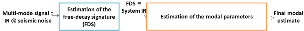
Figure 2.3: The general overview of the two steps of the output-only modal analysis.
