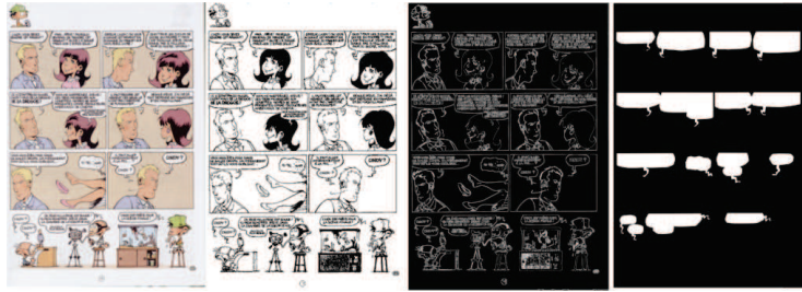
Figure 3.7: Balloon extraction process. Original image, binary segmentation, contour detection (connected components) and result mask from left to right. Image credits: [124].
