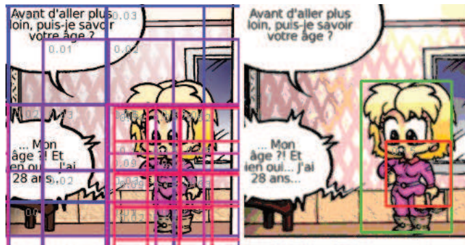
Figure 4.14: Multi-scale spotting example. The left image shows the detections at different scales, the colouration depends on to the p value, blue to red for low to high. The right side image shows the remaining best detection after the filtering step. Image credits: [37].
