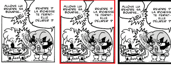
Figure 6.8: Implicit balloon recovery by closing open panels. From left to right: original panel, panel bounding box detection, panel with artificial frame from its bounding box that closes two balloons. The implicit balloons are now regular (closed).
