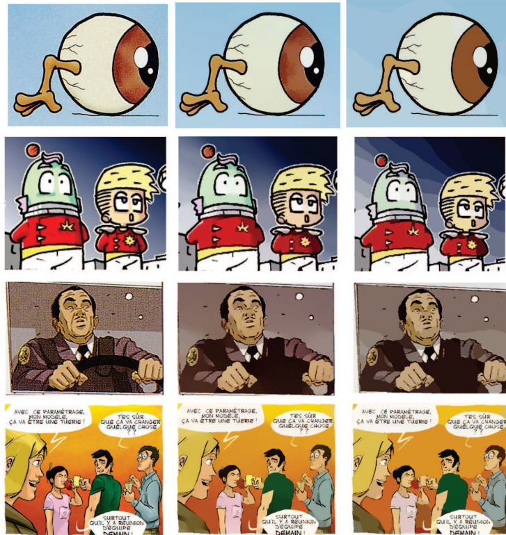
Figure 4.10: Colour image smoothing and quantization effects for comic character extraction. From left to right columns: original image, smoothing [201] and k-means clustering ( N = 32 ). Image credits: [37, 77, 94, 107].
