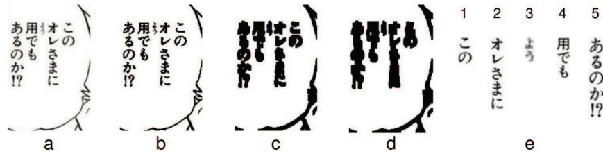
Figure 6.5: Sample of text extraction process. (a) Original balloon text image; (b) Threshold; (c) Morphology-Erosion filter; (d) Morphology-Opening filter; (e) Extracted blob from original image. Image from the original paper [8].
